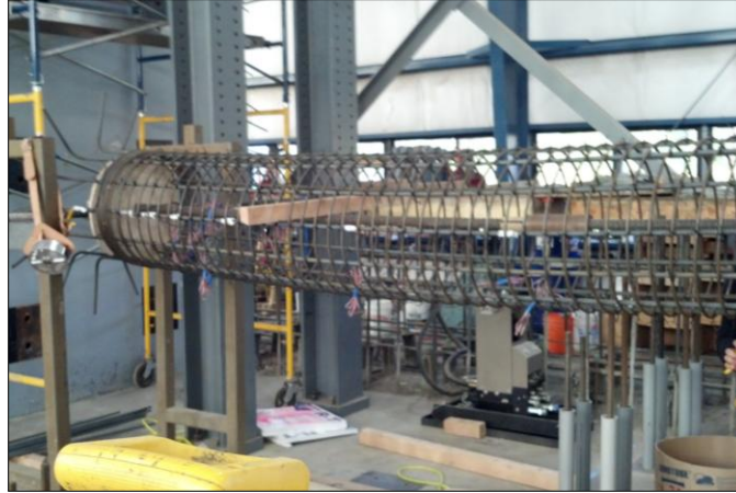
Figure 3.20 Photograph of Column C2 rebar cage
