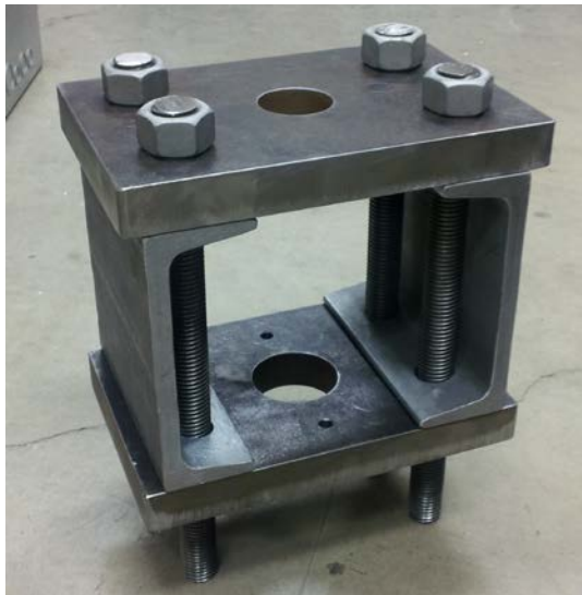
Figure 4.2: Universal Test Machine Adapters for 1.5 inch Anchor Rods
