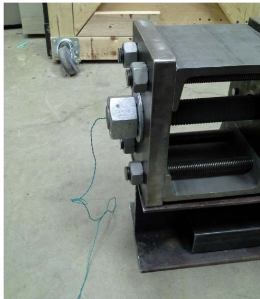
Figure 4.5: Direct Tension Indicator (DTI) Washer Calibration
