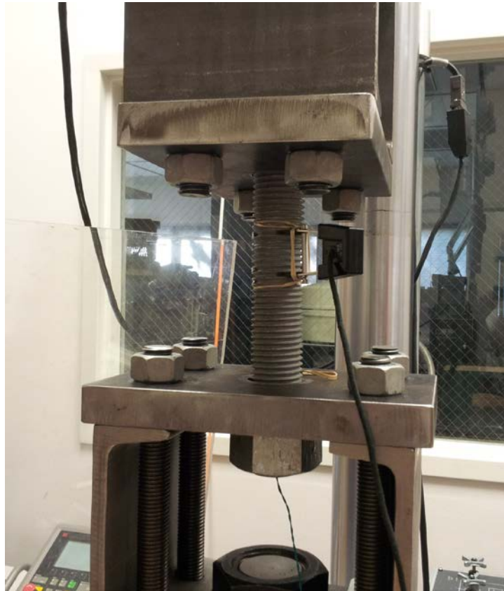
Figure 4.3: Anchor Rod Calibration in Universal Testing Machine
