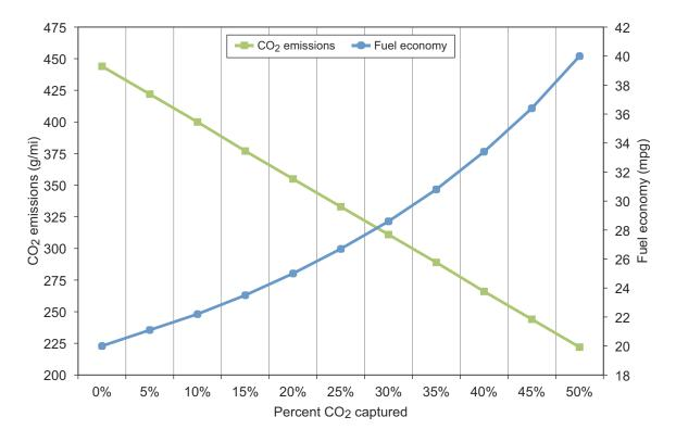
Figure 1.  $CO_2$  emissions and fuel economy at various levels of carbon capture (using 20 mpg as the baseline fuel economy value at 0% captured).
