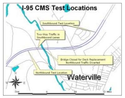
more caution on the northbound lane due to the need to maneuver through a lane cross-over. This fact lessened the need for additional warning signs on that approach. The CMS was placed at the end of a tapered section where barrels were used to close the left lane. Beyond that point the left lane carried the diverted northbound oncoming traffic. The following photographs show the traffic control measures and different perspectives of the experimental installation.
