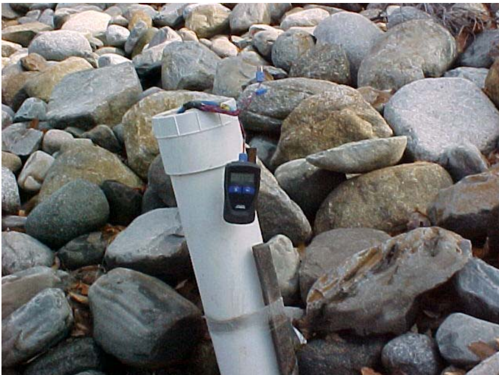
Figure 5. Digital Thermometer Connected to Thermocouple Leads
