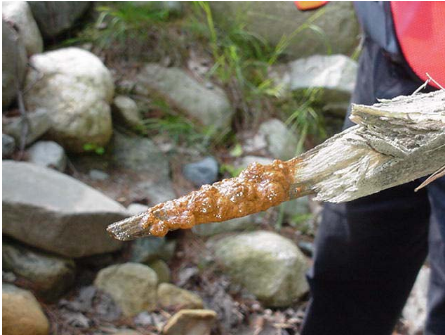
Figure 21. Surface Deposits Caused by Iron Bacteria
