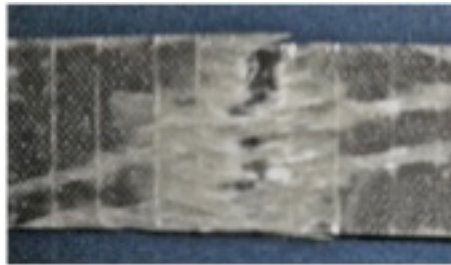
Figure 4.5 E-Glass Fiber Rupture Failure
