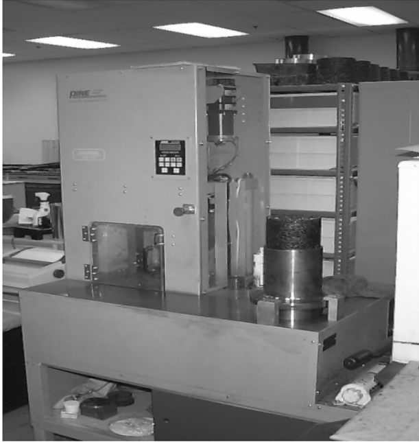
FIGURE 3.10: Compaction of Test Specimens Using the Superpave Gyratory Compactor
