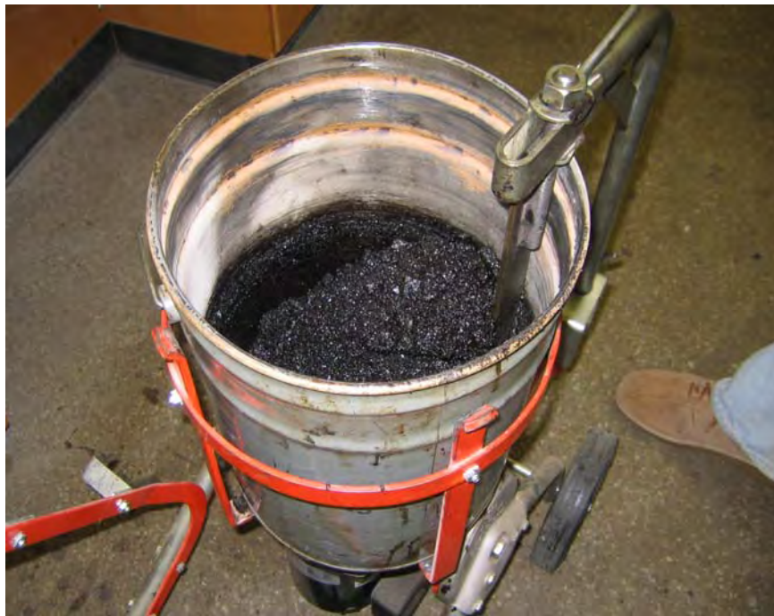
FIGURE 3.9: Mixing of Asphalt Binder and Aggregates in the Laboratory
