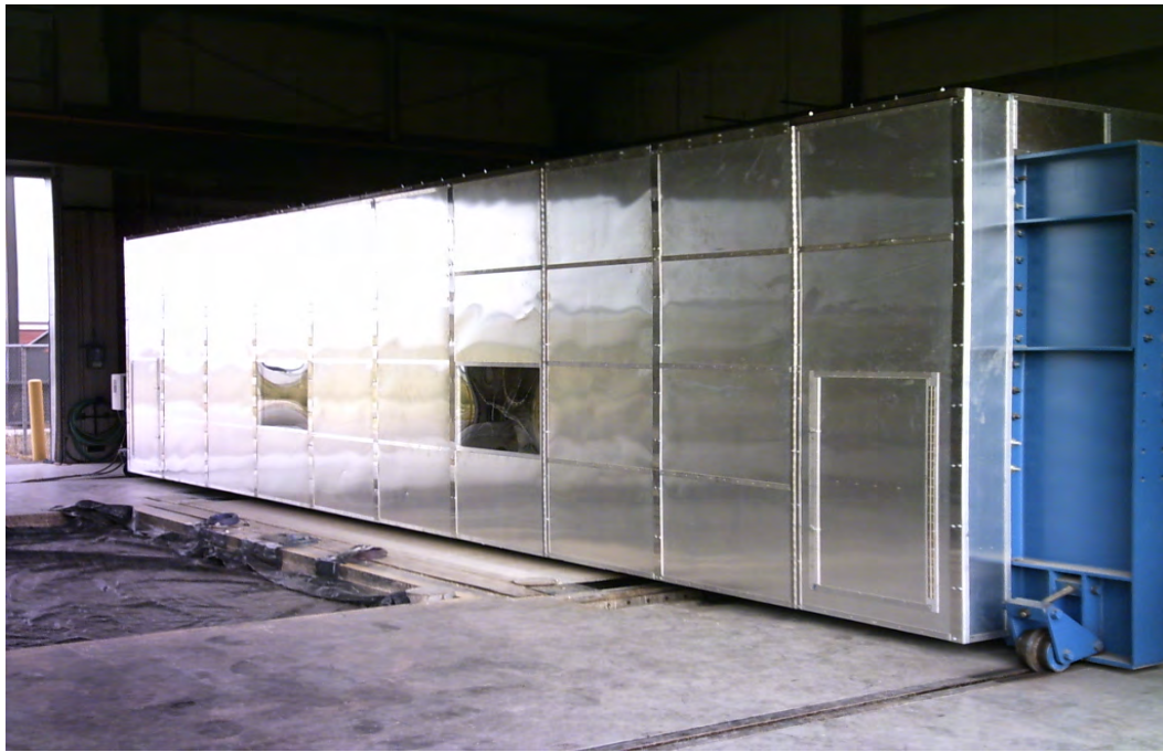
FIGURE 1.4: Accelerated Pavement Testing Machine with Temperature-Control Chamber
