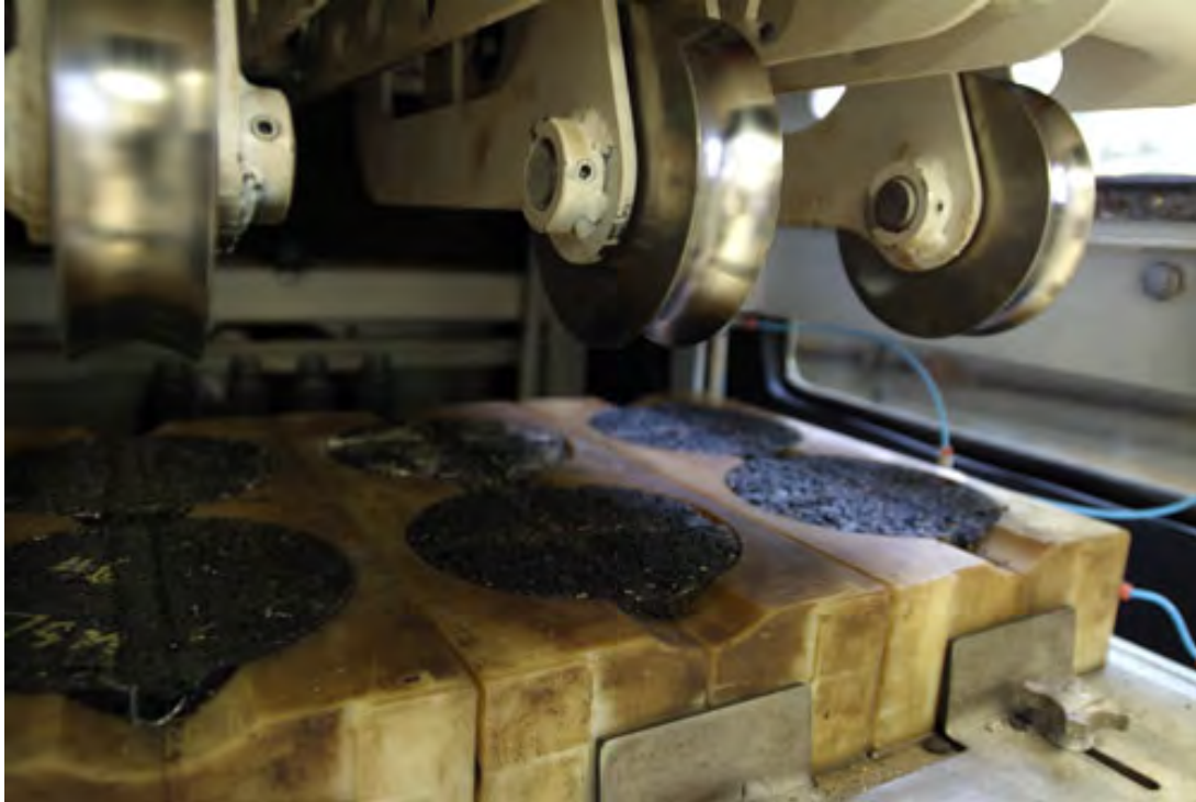
FIGURE 3.22: Asphalt Pavement Analyzer Test
