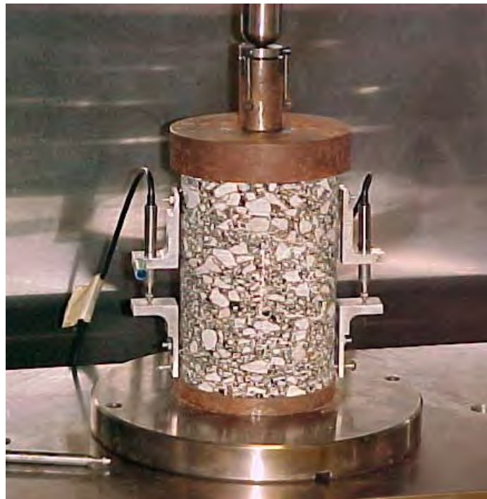
FIGURE 3.15: Sample Setup with Attached LVDTs
