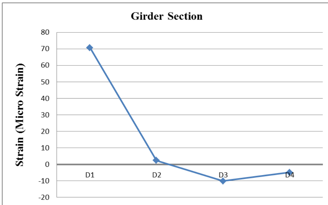
Figure G12. Girder D Strains For Maximum Positive Moment.
