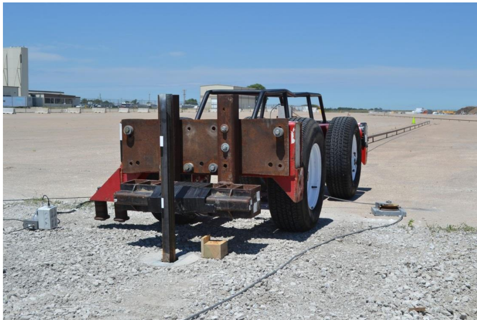
Figure 13. Rigid-Frame Bogie on Guidance Track
