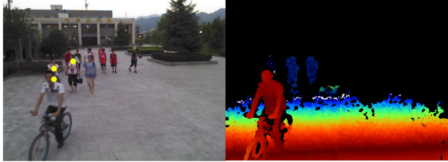
Figure 4.2 Example of missing detection (Yellow solid circle locating one pedestrian), RGB image on the left while corresponding depth image on right
