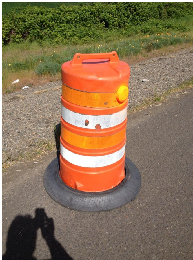
Figure 5.1 DCU deployed on I-5 for origin-destination data collection
