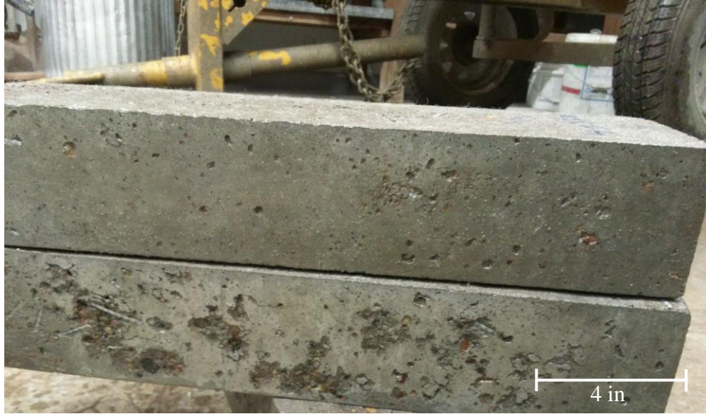
Figure 4.15: FHPC D7.5 specimens after 300 cycles
