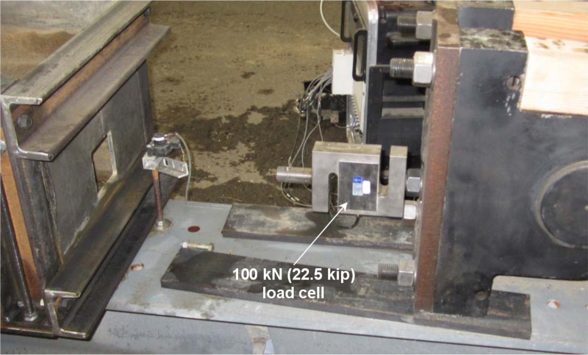
Figure 0.4 Load cell used for the majority testing (looking east).
