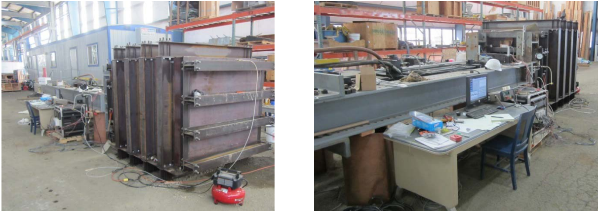
Figure 6.3 Photos of the multi-strip pullout box assembly.
