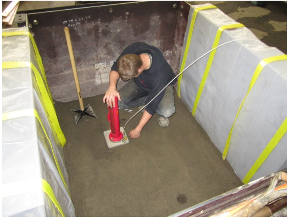
Figure 6.7 Balloon density gage testing.
