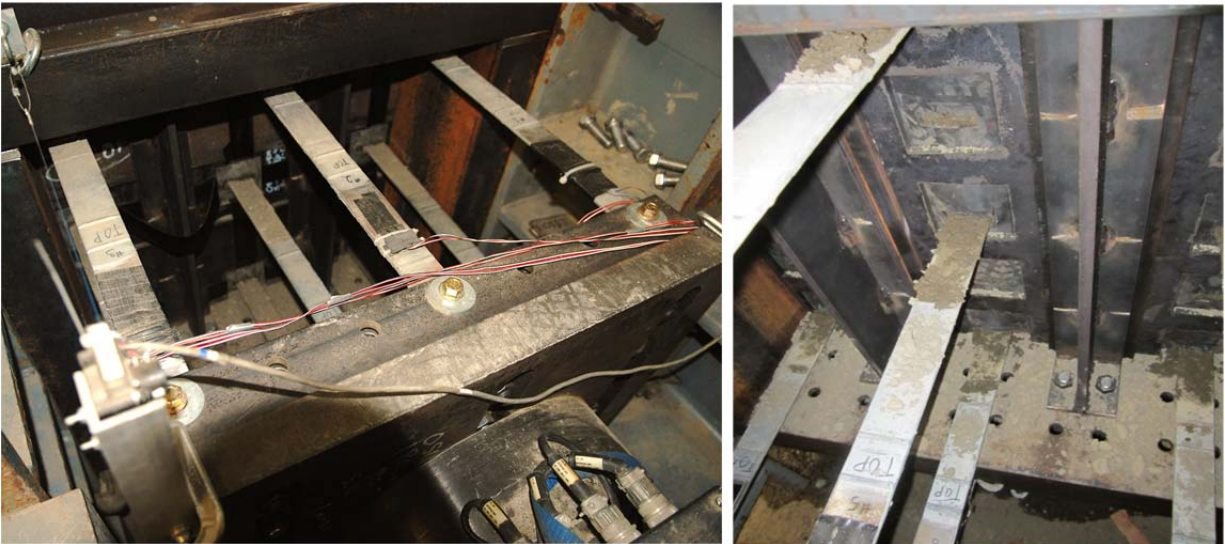
Figure 6.5 View of reinforced front panel section during test.
