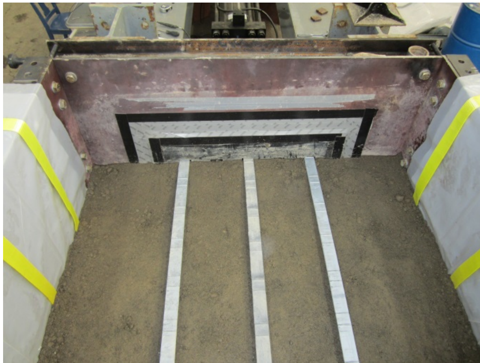
Figure 6.8 View of reinforcement strips placed on a compacted lift of fill soil.
