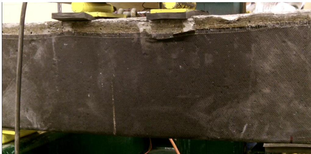
Figure 8: 254 mm Deep Beam, B2, No Grooves, after Failure
