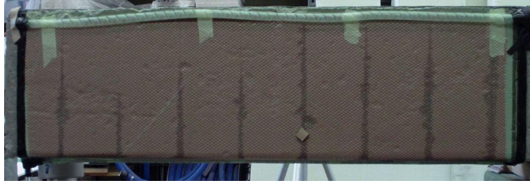
Figure 4: VARTM, Beam 1 with 3.2 mm Grooves, 30 sec
