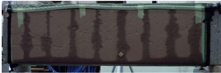
Figure 5: VARTM, Beam 1 with 3.2 mm Grooves, 60 sec
