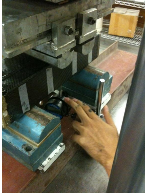
Figure 6: Strength Test - Deflectometer
