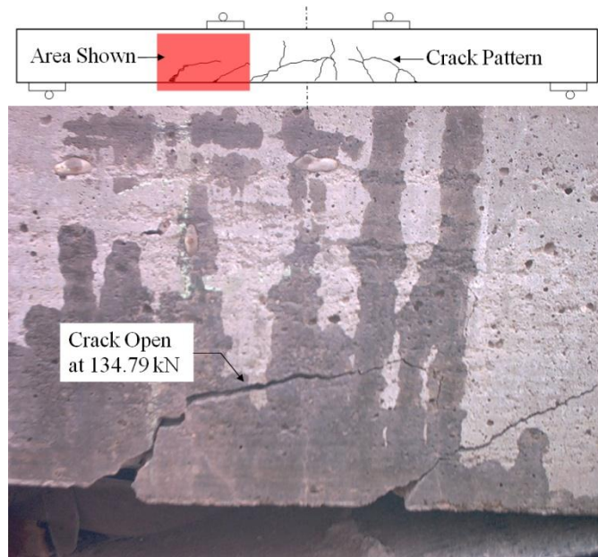
Figure 10: Flexural Hand Layup Beam
