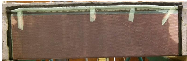
Figure 9: VARTM, Beam 2 with 6.4 mm Grooves, 342 sec
