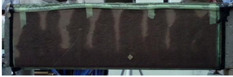
Figure 7: VARTM, Beam 1 with 3.2 mm Grooves, 120 sec
