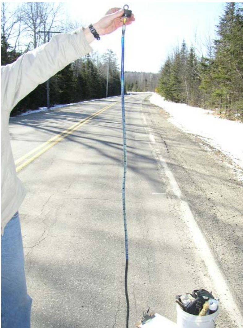
Photo 1: Frost Gauge Reading on 3/21/2007. Blue dye is visible at the top and bottom of the gauge (unfrozen state). Clear section is frozen.
