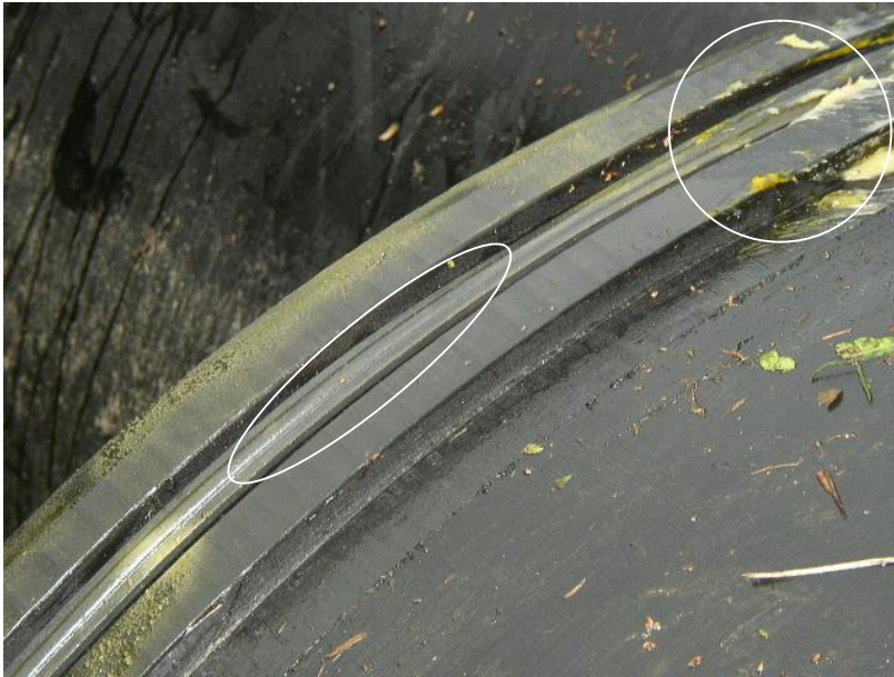
Figure 3 O Ring seal on male end of Snap-Tite Pipe. A small amount of pipe lubricant can be seen in the upper right corner.
