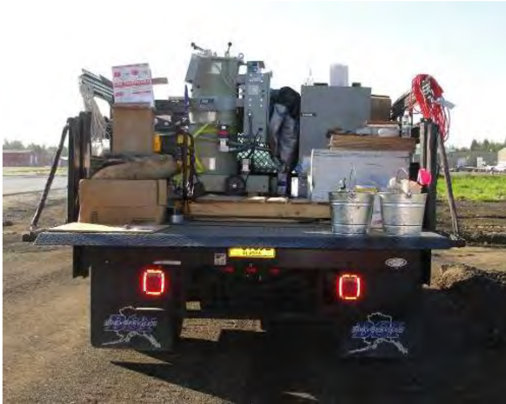
Figure 3.2 Field lab for AIA paving project
