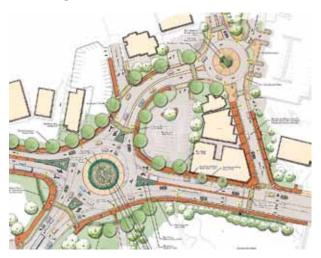
The roundabouts at the Hillsborough/Pullen (lower left) and Oberlin/Pullen (upper right) intersections reflect the variety of design options available in just this one type of intersection. Higher-volume, multi-lane roadways can still be accommodated with roundabouts through the use of two lanes in the circulating roadway.
