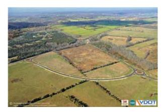
Along VA Route 50, the Gilberts Corner roundabout plan accommodates substantial turning movements between Route 50 and Route 15 by adding a new diagonal connecting road with additional roundabouts.
