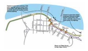
Recommended changes to Riverfront Parkway included the addition of access to downtown Chattanooga through new at-grade intersections and, in some places, the reduction of roadway width from four to two lanes. Designers made a case that the use of network preserved overall system capacity but that the re-design of the Parkway restored riverfront access from downtown.
