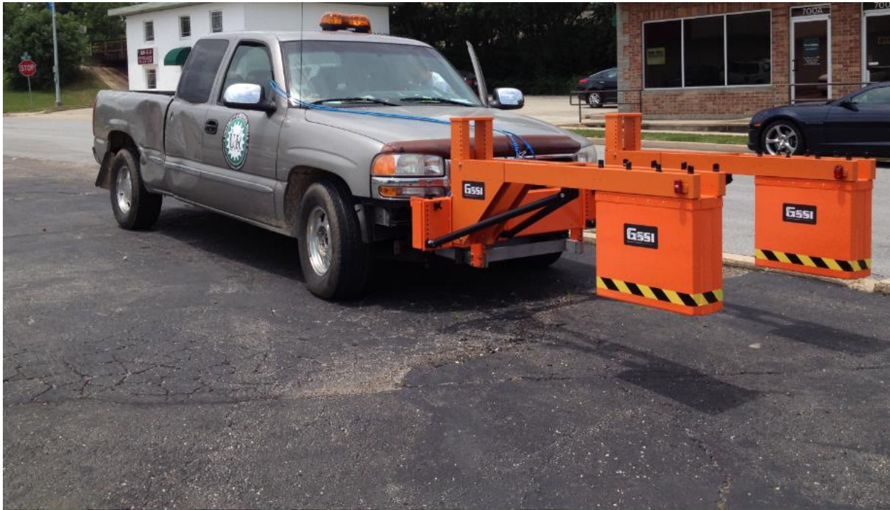
Figure 3-1 Photo of 2.0 GHz GSSI Antennae Mounted to Vehicle
