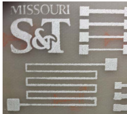
FIG 12: Results of patterning with screen-printing on FR4.
