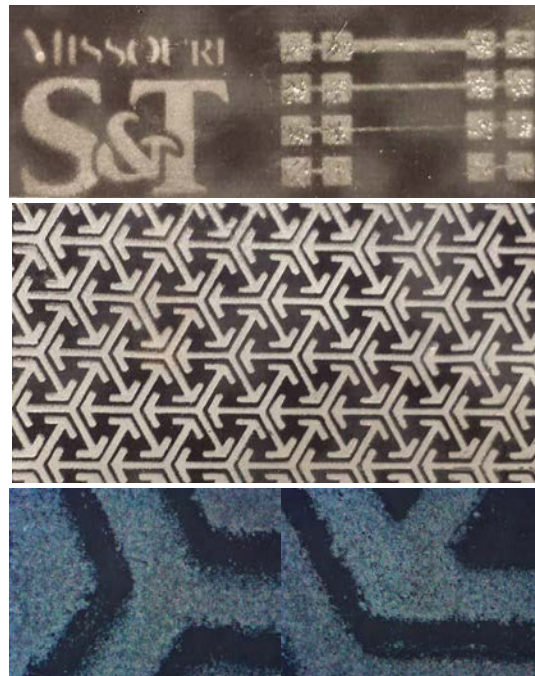
FIG 11: Results of patterning with stencil and air-brush on Duroid
