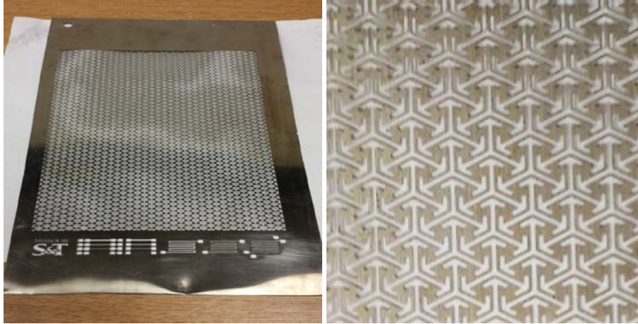
FIG 10: Photograph of stencil used with air-brush.
