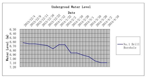
Figure 8: Underground water level in Borehole 1.
