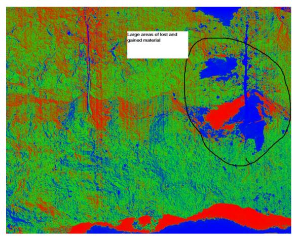
Figure 15: Initial results of change detection algorithm. Gained material is shown in red, and lost material is shown in blue. Note that tree in Figure 14 has been removed. The bottom of the image shows fallen rock.
