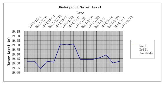
Figure 8: Underground water level in Borehole 2.
