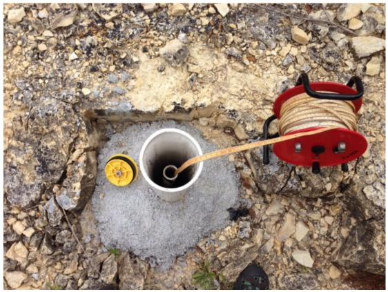
Figure 7: Making water level measurements.
