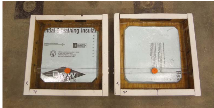
a) Molds and RFID Sensors' Installation Detail
