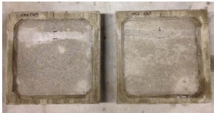
b) Ponding Test Specimens after Removing the Molds
