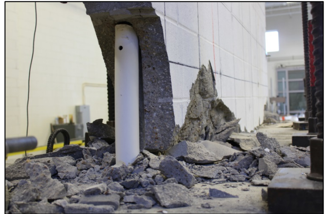
Figure (49): The general mode of failure for wall 3
