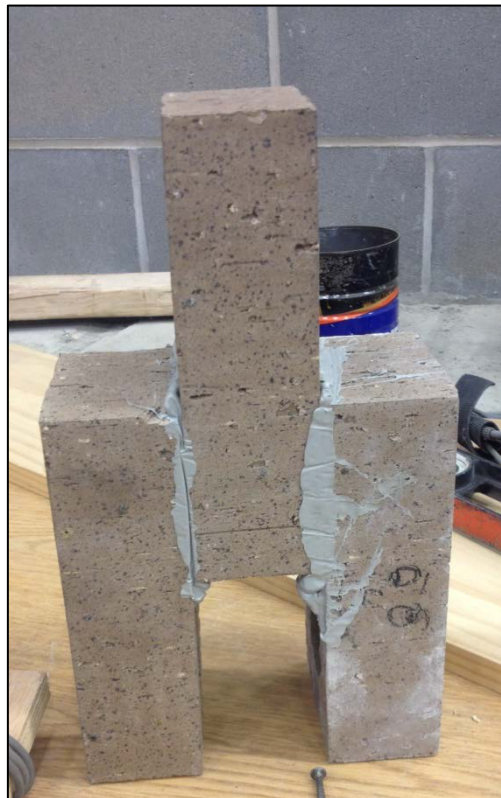
Fig (14): Testing the adhesion of the epoxy
