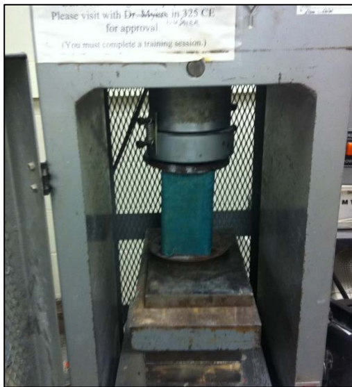
Figure (22): Grout testing
