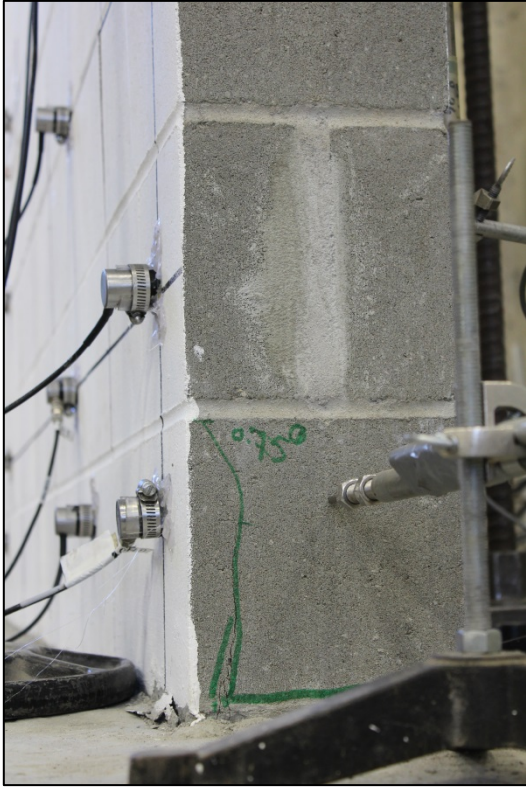
Figure (43): The first crack in the toe at 0.75 inch displacement
