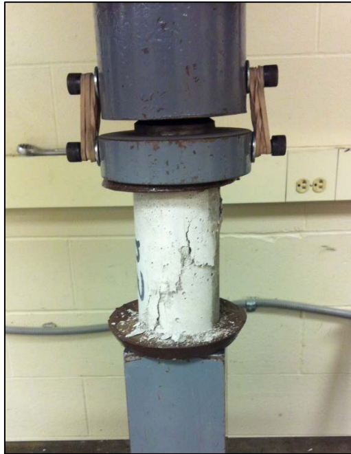
Figure (21): Mortar testing
