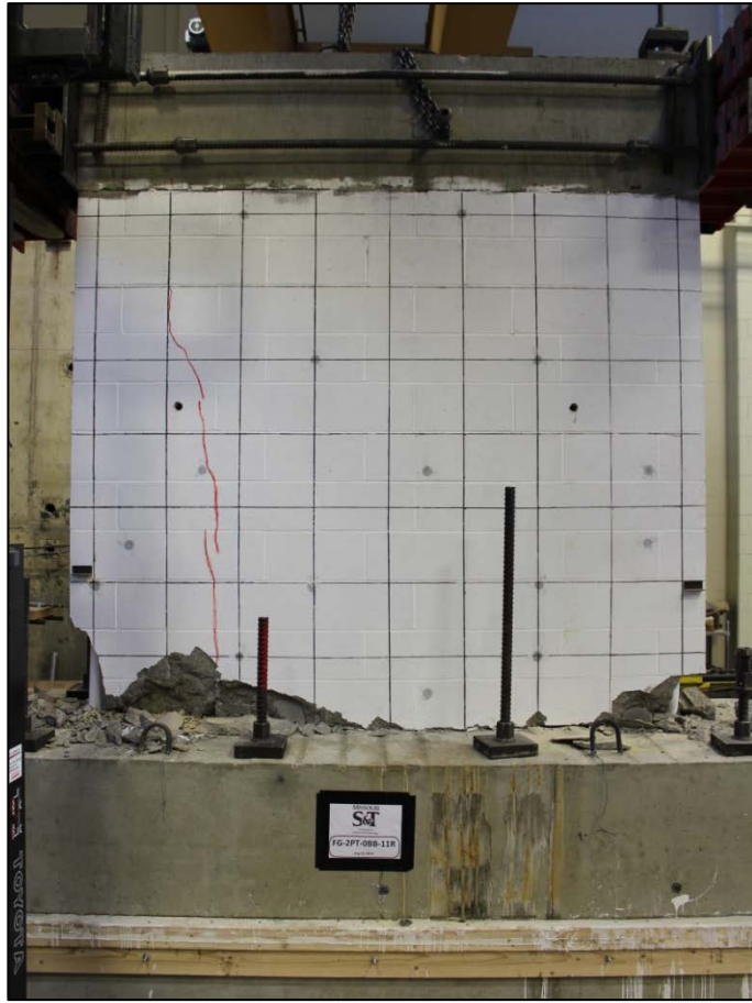
Figure (49): The general mode of failure for wall 3
