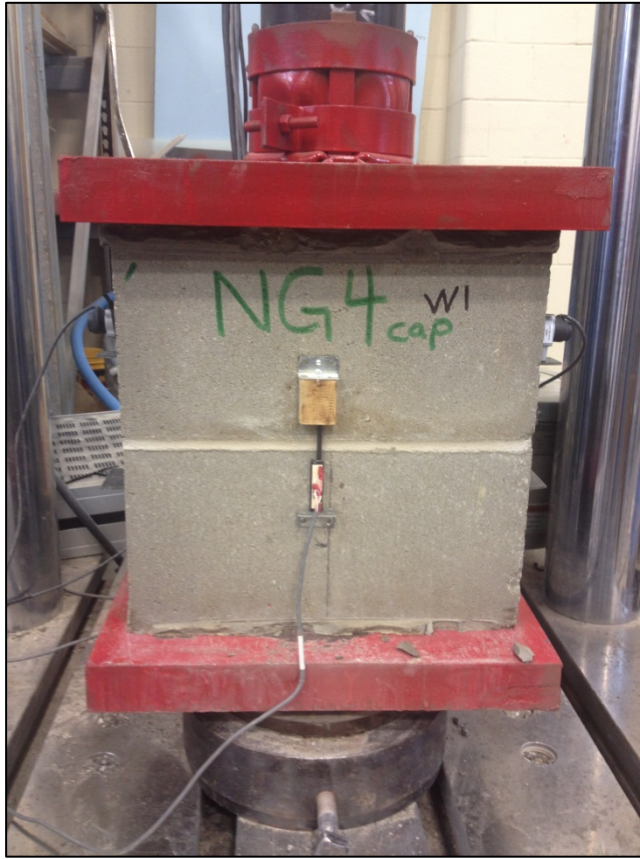
Figure (23): Masonry block prism test
