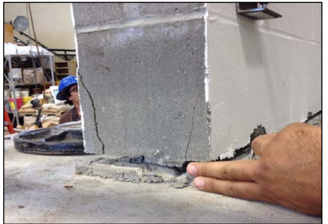
Figure (51): Cracks developing in the toe of wall 3
