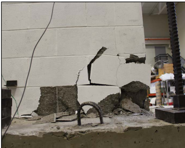
Figure (42): The toe failure for wall 2
