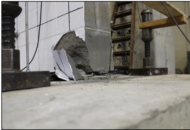
Figure (51): Cracks developing in the toe of wall 3
