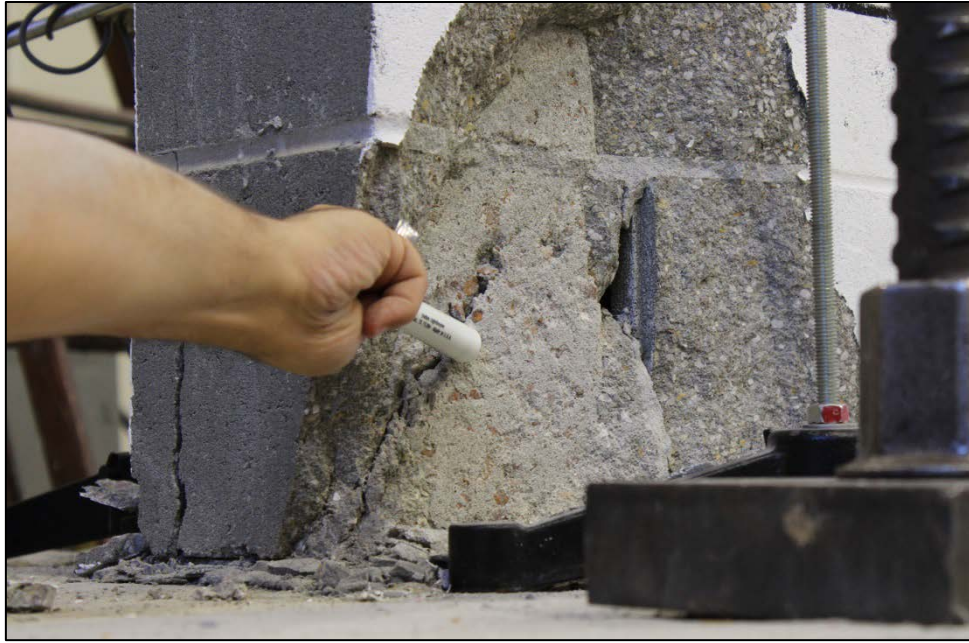
Figure (44): Developed toe crack
