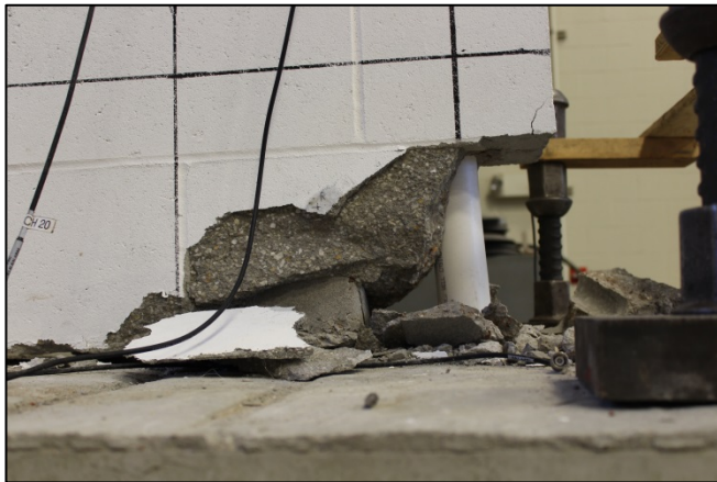
Figure (49): The general mode of failure for wall 3
