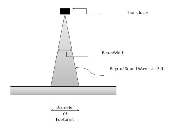
Figure 12: Illustrates the transducer beamwidth (Modified after Mueller & Landers, 1999).
