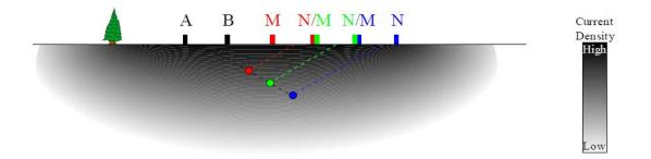
Figure 13: Multi-electrode dipole-dipole resistivity array (Frontier Geosciences, 2001).
