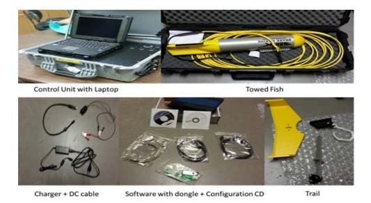
Figure 21: Side Scan Sonar (Yellowfin) Model 872.
