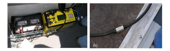
Figure 23: Equipment Photos (a) AGI Supersting Marine (b) stainless steel electrode on towed cable. (Enviroprobe Service, Inc.).
