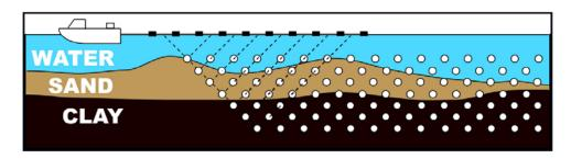
Figure 14: Sample setup of marine survey an array of electrodes towed behind a boat (Wei, 2011).
