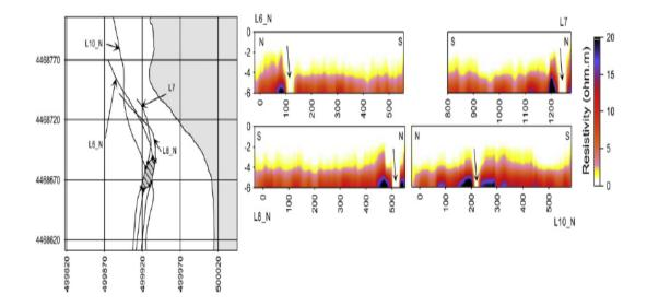
Figure 15: Navigation map and "picking" of the coordinates (latitude and longitude) corresponding with low resistivity anomaly in inverted resistivity profiles. Asterisks in the A frame correspond to the vertical stripes detected in four profiles (indicated arrows). The union of these points (filled polygon in leftmost frame) defines an area having an extension of about 25/30m along NE-SW,and13-15m along NW\_SE. Datum isWGS84, projection is UTM (Zone33) (Passaro, 2007).
