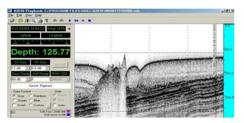
Figure 19: The sub bottom profiler and bathymetric acquisition software.
