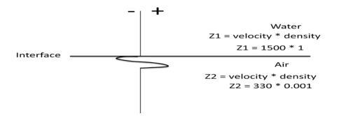
Figuer 9: The reflection coefficient of the interface between water/Air is -1.0.
