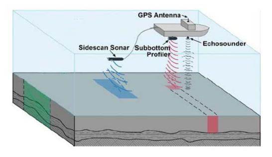
Figure 8: Acoustical geophysical methods for over-water surveys. (Modified after Savini, 2011).
