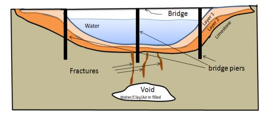
Figure 2: A sketch of bedrock fractures that may make the bridge piers unstable.
