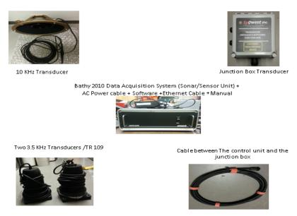
Figure 18: Bathy 2010PC<sup>TM</sup> CHIRP Sub Bottom Profiler and Bathymetric components.
