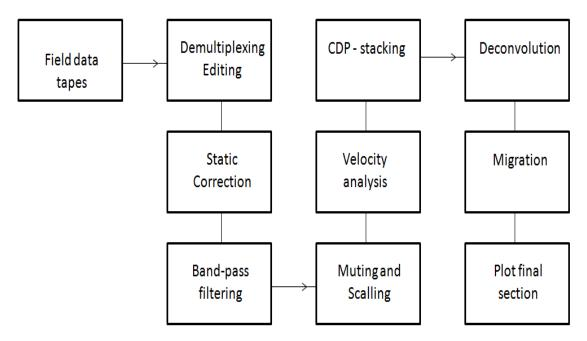
Figure 22: An overview of reflection seismic data processing. Data-processing flow is usually tailored to handle the requirements and problems of the individual data-set (Sharma, 1997).
