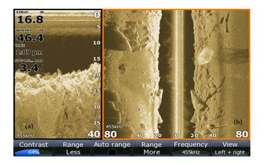
Figure 20: StructureScan HD data (a) downscan data, (b) side scan sonar imaging (Lowrance, Inc).
