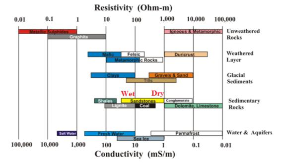
Figure 5: Typical ranges of electrical resistivity (ohm-m) or conductivity (mS/m) for selected Earth materials (Palacky 1988).
