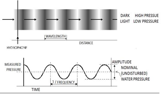
Figure 6: Components of a Sound Wave (Vaduva, 2000).
