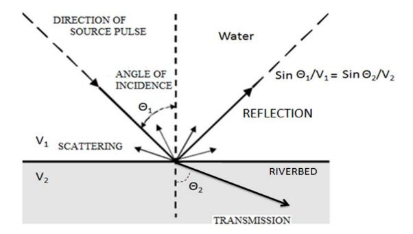
Figure 7: Components of an Echo Event on the Ocean Floor (Modified after Vaduva, 2000).
