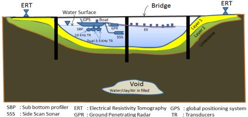
Figure 16: A simple model shows a demonstration of all geophysics surveys over water.
