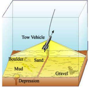
Figure 11: shows side scan sonar (Kvitek et al., 1999).
