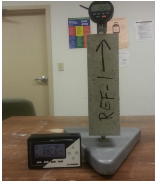
Figure 4-1. Photo of length measurement for drying shrinkage
