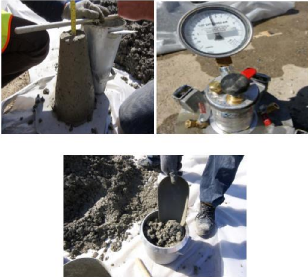
Figure 5-5. Photos of fresh property testing at job site
