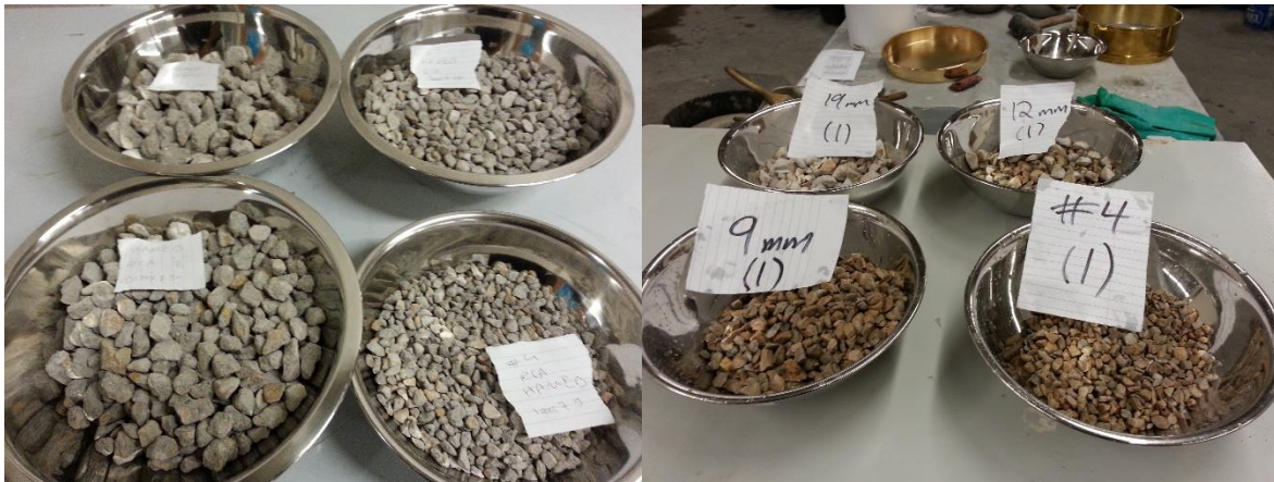
Figure 3-1. RCA particles before separating the mortar (left) and after separating the residual mortar (right)
