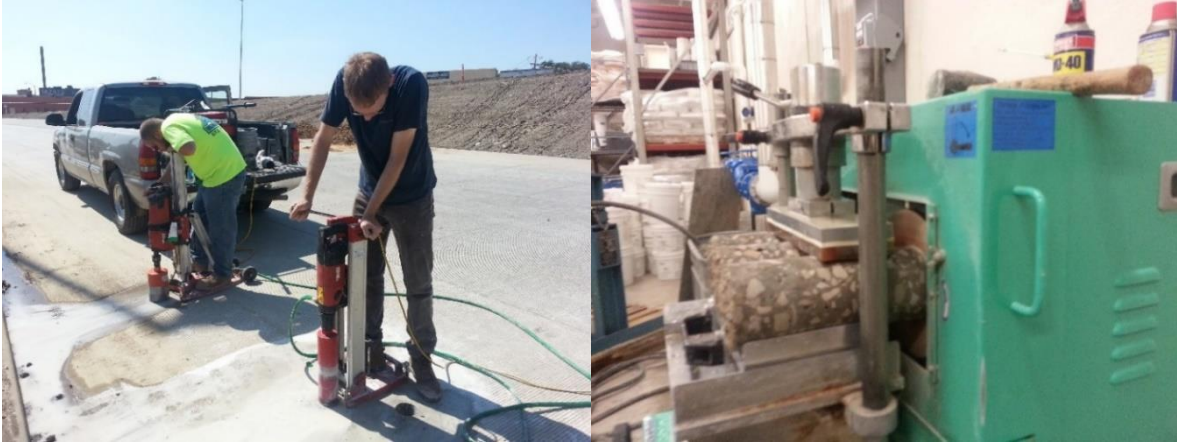
Figure 5-16. Photos of core sampling at the job site (left) and grinding the test surface of the specimens (right)
