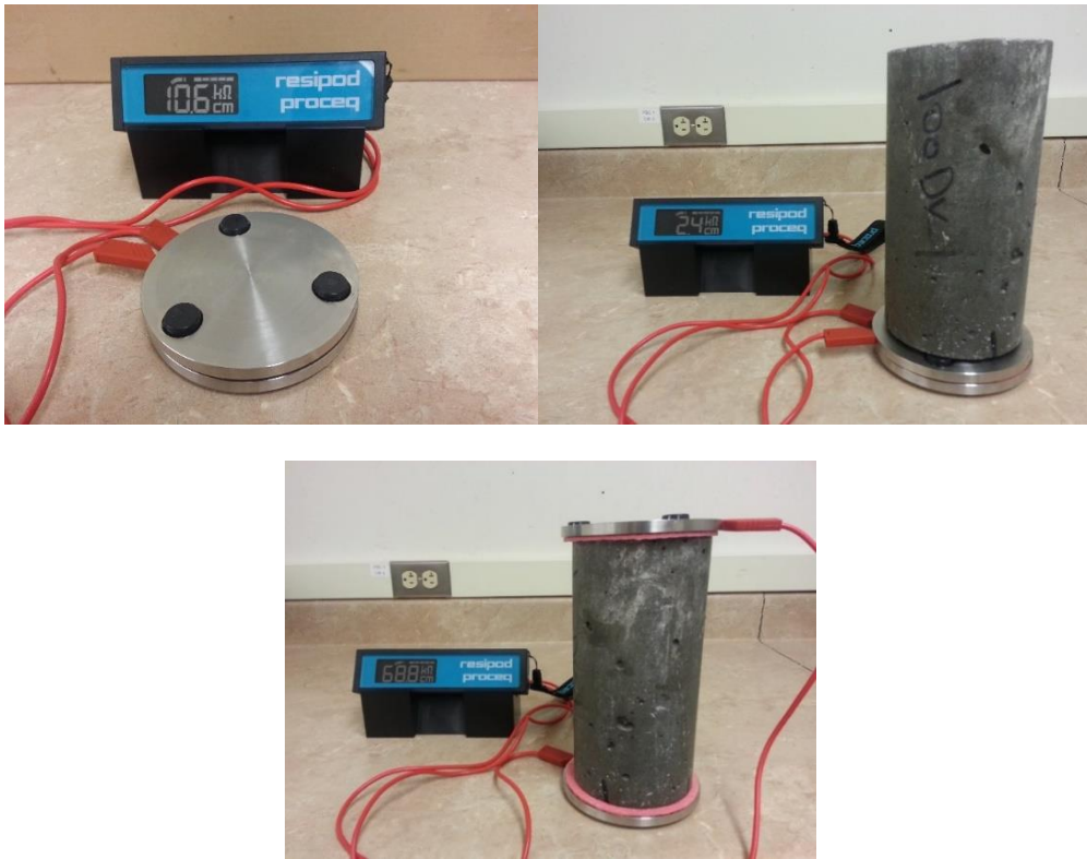
Figure 4-14. Measuring bulk electrical resistivity
