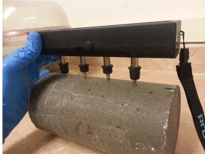
Figure 4-12. Surface resistivity measurement
