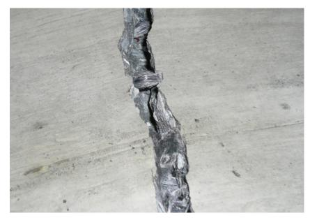
Figure 4.14: Carbon Fiber Bridging Crack along Bottom of Panel
