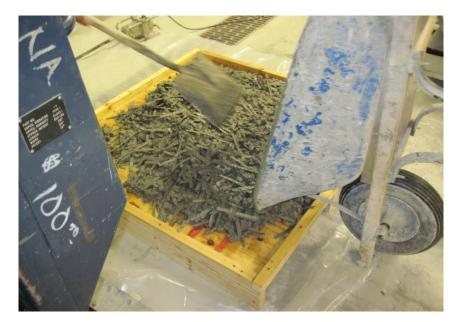
Figure 4.3. LCFRC Impact Panel Construction
