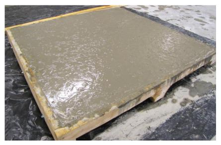
Figure 4.4. Completed LCFRC Impact Panel In Formwork
