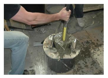
Figure 3.1. ASTM C995 Fiber- Concrete Flow Cone Test
