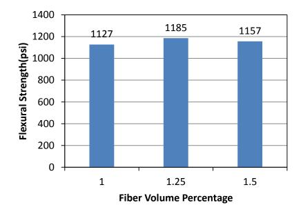
Figure 3.3. Flexural Strength Test Results (ASTM C78)
