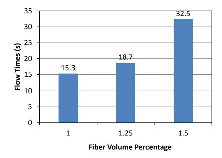
Figure 3.2. Flow Cone Test Results (ASTM C995)
