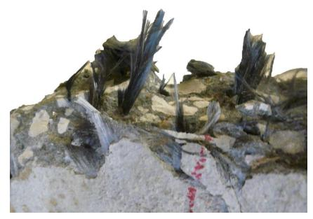
Figure 4.15: Carbon Fiber Pullout from LCFRC Panel Impact Test
