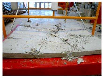
Figure 4.11: Typical Top of WWR Panel Failed Specimen
