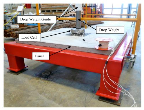
Figure 4.5: Drop-Weight Impact Test Setup
