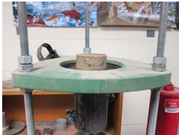
Figure 14 – Sample being extruded
