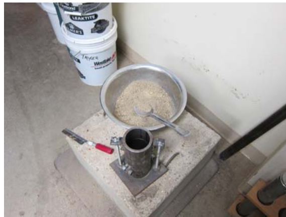
Figure 10 – Compaction equipment and soil
