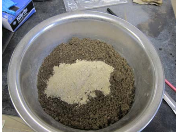
Figure 8 – Soil and additive combined prior to mixing
