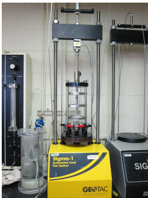
Figure 26 – Load Frame used to perform unconfined compression strength measurements
