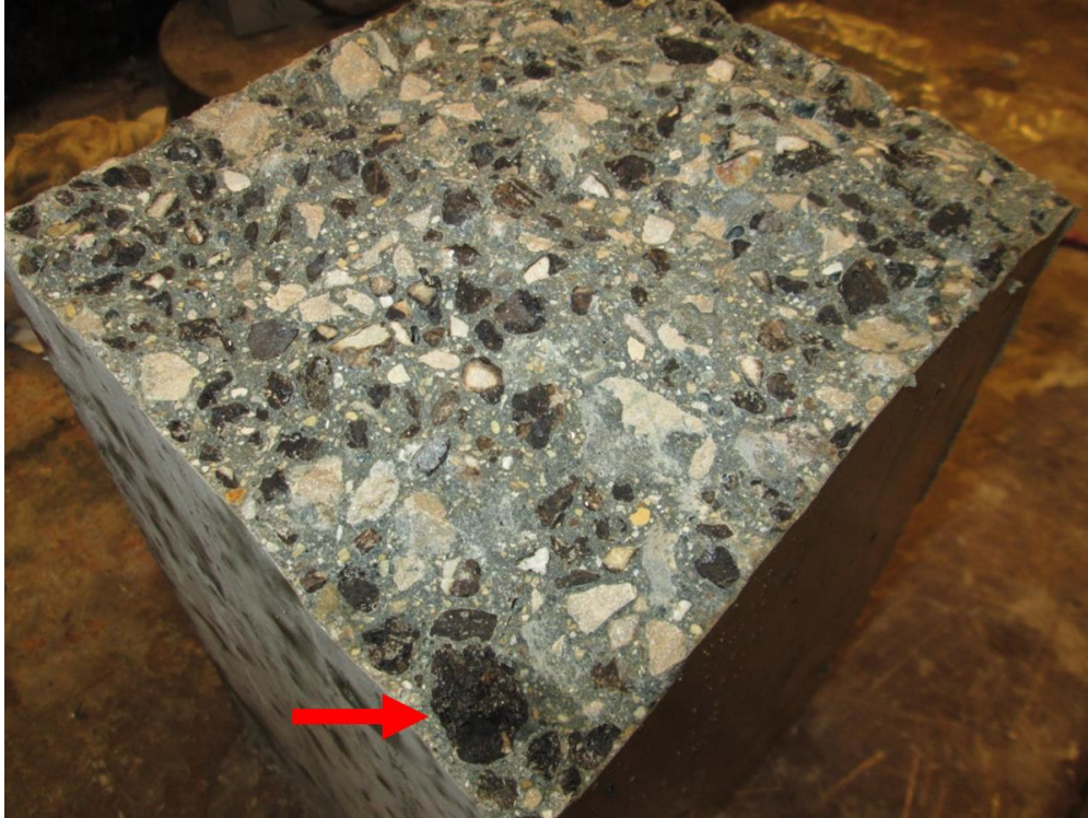
Figure 58. An image of one of the flexural strength beams where a large agglomerated FRAP particle appeared to affect the path of the crack.
