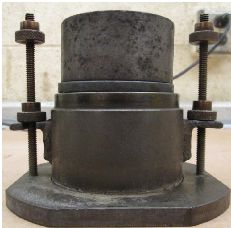
Figure 39. SFS FRAP 3 (Central Blacktop) exhibited little to no expansion after autoclaving.
