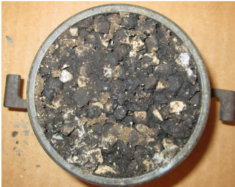
Figure 38. The base of the mold after autoclaving contains a significant amount of agglomerated asphalt.
