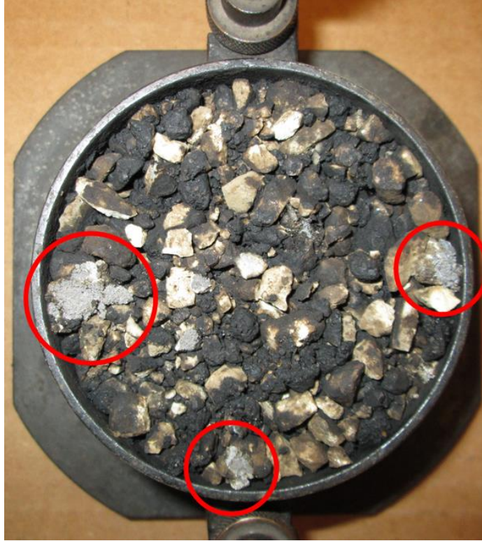
Figure 37. The SFS particles in the FRAP that disintegrated are circled, which is evidence of the \beta -dicalcium silicate (larnite) to \gamma -dicalcium silicate (calcio-olivine) phase transformation.
