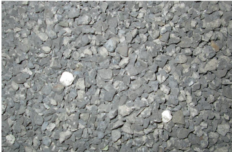
Figure 20. Particles of unassimilated CaO (white particles) could be seen in the Virgin SFS 1 (BOF) sample after crushing.
