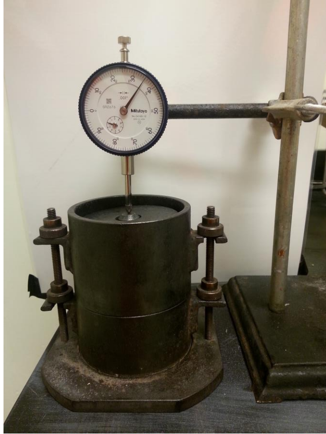
Figure 36. Measurement of the height of autoclave expansion mold.
