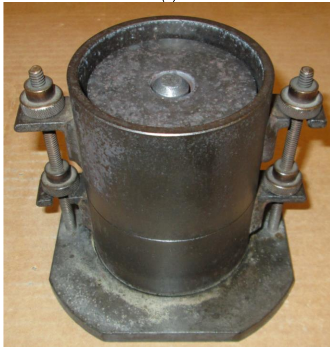
Figure 35. Components (a) and completed assembly (b) of the autoclave expansion mold.
