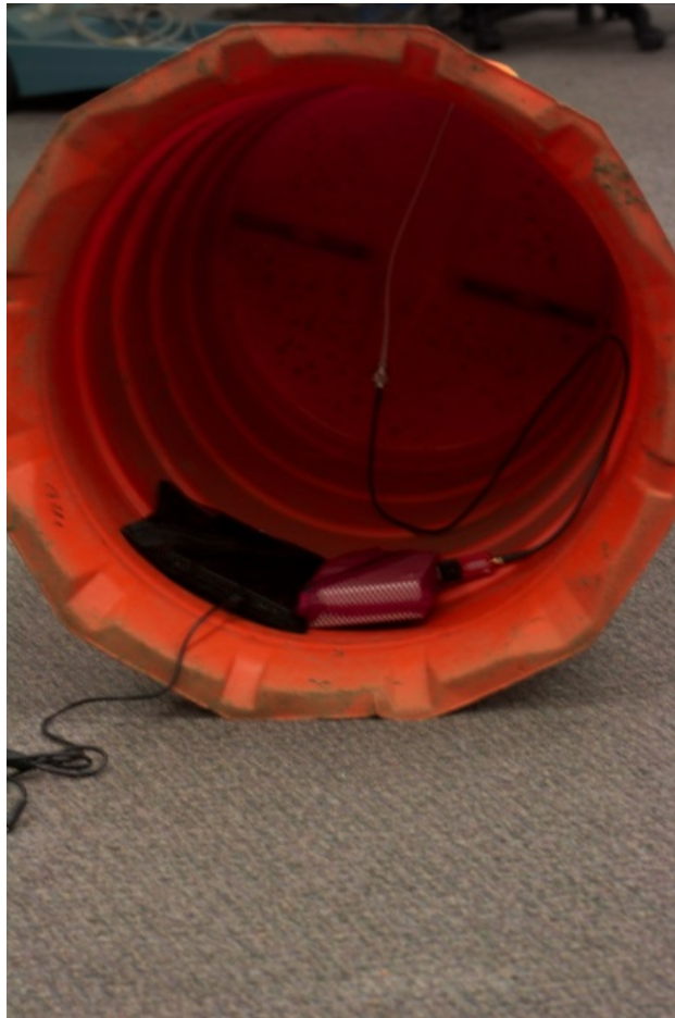
Figure A.4: DCU and battery in pouches and clipped to O-rings mounted on the inside of the traffic barrel.
