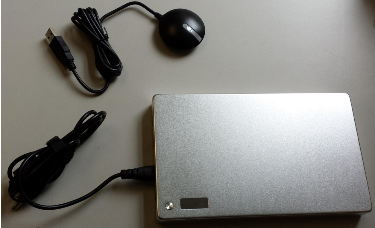
Figure 3.4: Battery and GPS module
