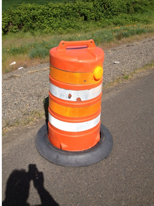
Figure 3.7: DCU deployed on I-5 for origin destination data collection
