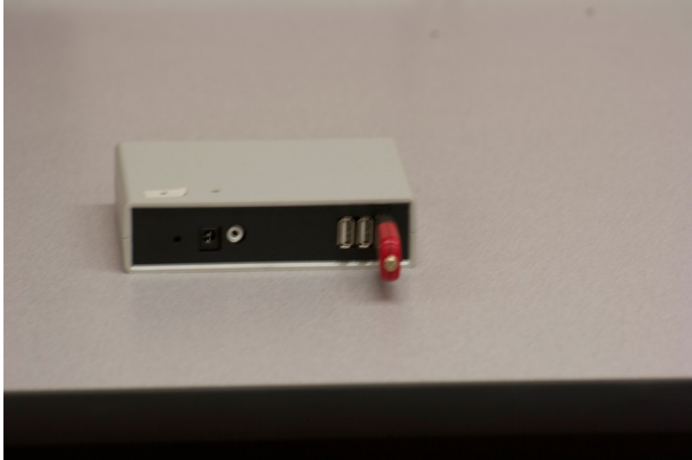
Figure A.5: External Bluetooth module mounted to the first USB port on the DCU
