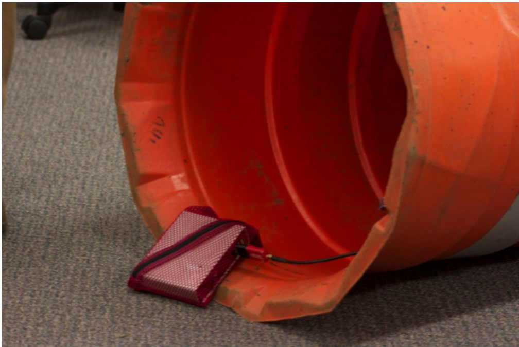
Figure A.6: Connection of the antenna cable extension to the external Bluetooth module
