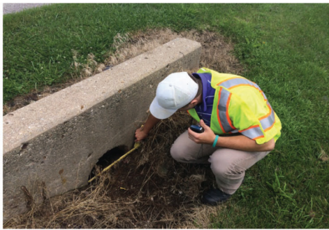
(c) Measuring span of culvert
