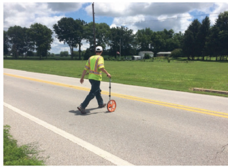
(d) Measuring the length of the culvert with a wheel
