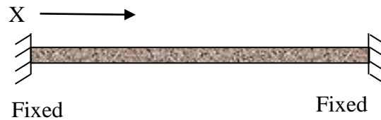
Figure 5-5: Beam with fixed end supports.
