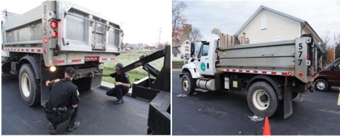
A: Measuring truck axle dimensions
