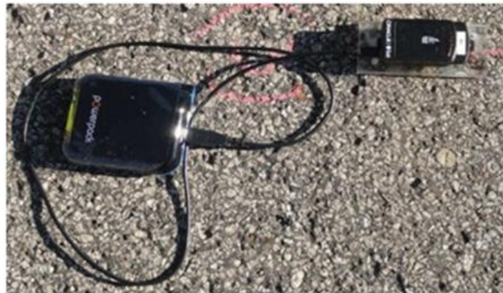
Figure 2-7: SunSPOT sensors with external battery.
