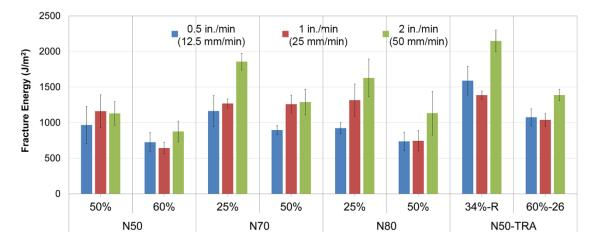
Figure 20. Fracture energy results from the SCB test conducted at 77°F (25°C) using LVDT control and varying rates 0.5 in./min, 1 in./min, and 2 in./min (12.5, 25, and 50 mm/min).
