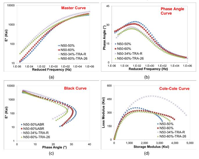
Figure 22. Viscoelastic characterization of the N50 mixes: (a) Master curve, (b) Phase angle, (c) Black curve, (d) Cole-Cole plots.
