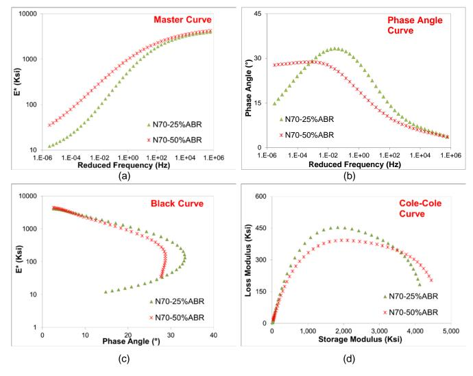
Figure 23. Viscoelastic characterization of the N70 mixes: (a) Master curve, (b) Phase angle, (c) Black curve, (d) Cole-Cole plots.
