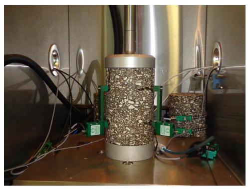
Figure 21. Complex modulus test specimen and fixture with axial extensometers mounted to measure deformations.
