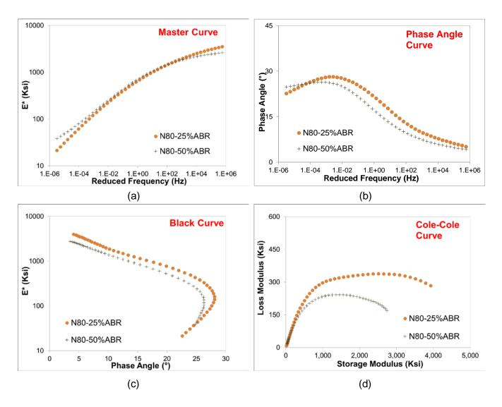
Figure 24. Viscoelastic characterization of the N80 mixes: (a) Master curve, (b) Phase angle, (c) Black curve, (d) Cole-Cole plots.
