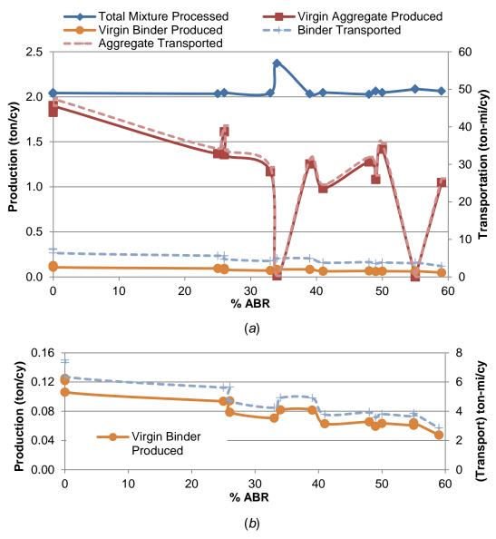
Figure 25. Quantities produced and transported per cy asphalt mixture for (a) all energy-intensive items and (b) only virgin binder, detailed.
