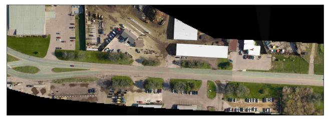
AeroMetric collected asset inventories on seventeen MDOT highway assets. Point assets include catch basins/drop inlets, crash attenuators, delineators, signs, sweepable approaches, and traffic signals. Linear assets include curbs, ditches, guardrail, concrete lane miles, bituminous lane miles, ROW fencing, and shoulders. Lastly, MDOT requested data on mowable acres.
