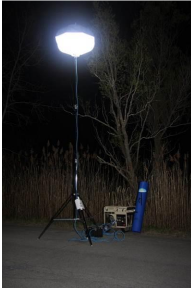
Figure 2-25. Balloon light (umbrella structure) with two 1000 W MH sources.
