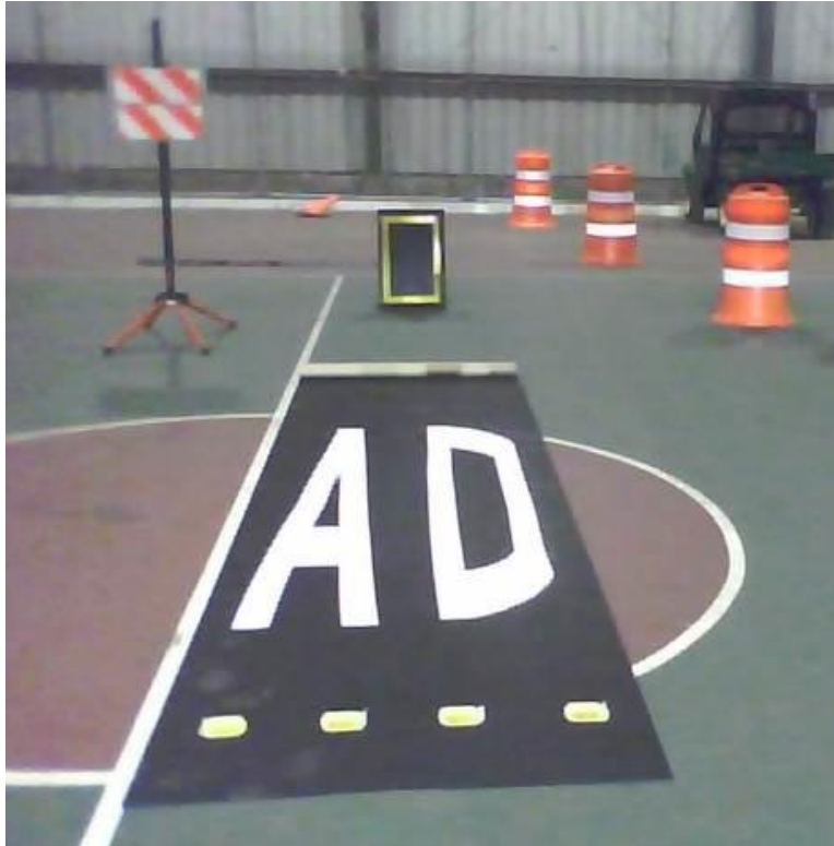
Figure 3-12. Barricade sheeting, reflective marker tape, wet reflective pavement letter symbols, raised pavement reflectors and traffic drums.
