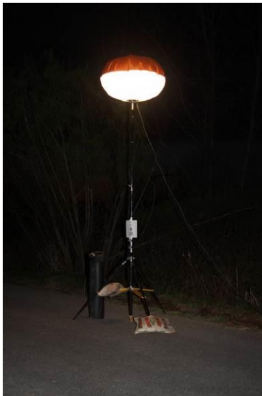
Figure 2-22. Balloon light (inflatable) with four 500 W halogen sources.
