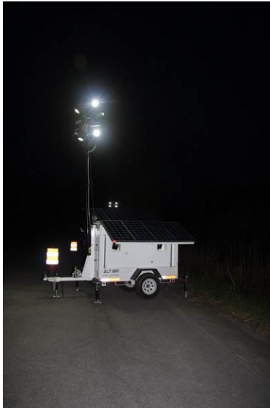
Figure 2-20. Solar-powered light tower with 1200 W LED lights.
