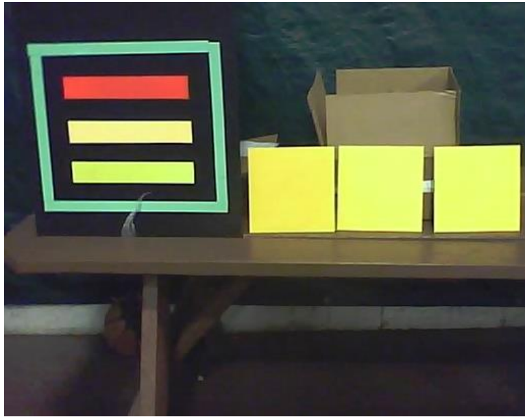
Figure 3-14. Photoluminescent tape materials (left) in various colors, and painted metal samples (right) of yellow color.
