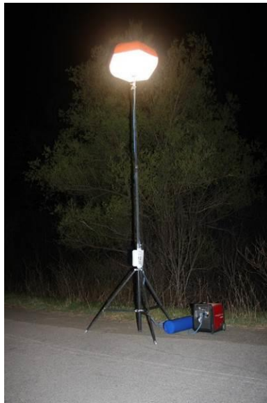
Figure 2-28. Balloon light (umbrella structure) with four 500 W halogen sources.
