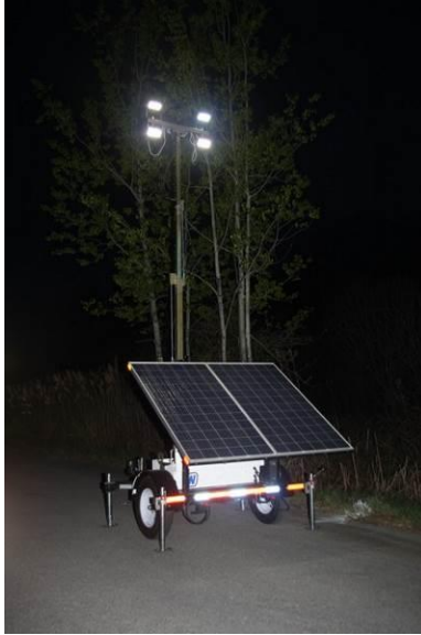
Figure 2-19. Solar-powered light tower with four 52 W LED lights.
