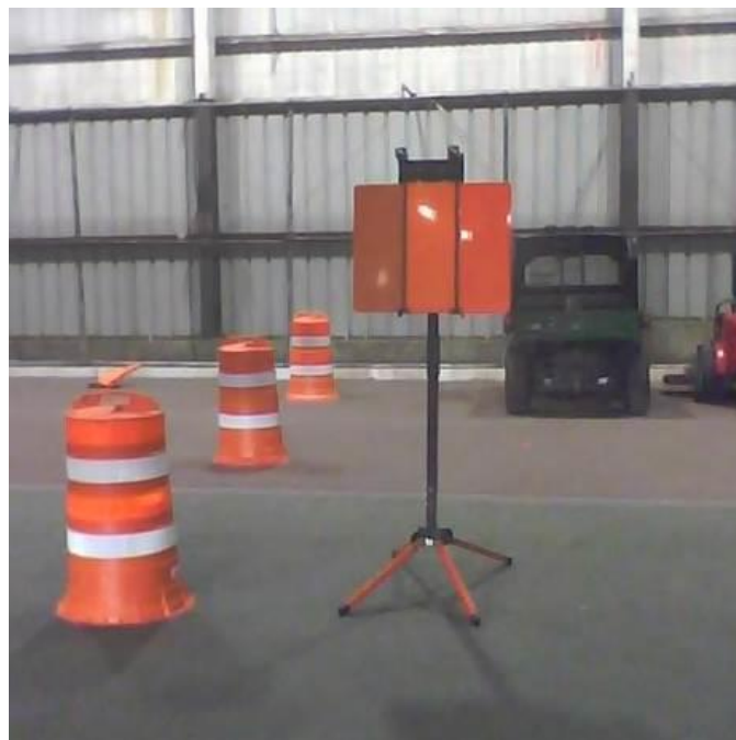
Figure 3-11. Traffic drums and orange reflective work zone sign panel containing three different sheeting materials.
