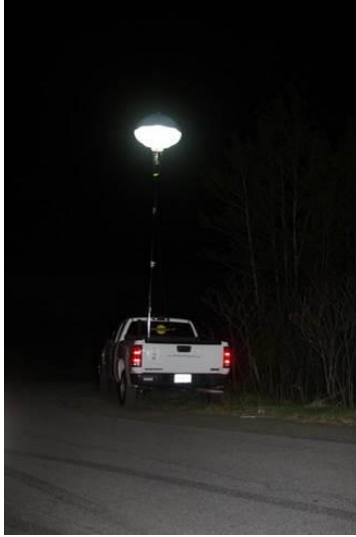
Figure 2-27. Balloon light (umbrella structure) with 700 W LED source.
