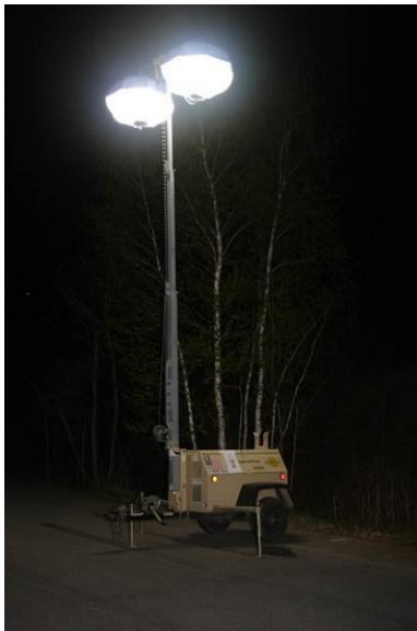
Figure 2-26. Balloon light (umbrella structure) with two 2000 W MH sources.
