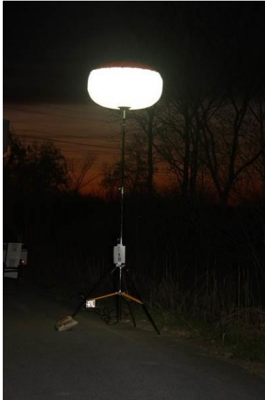
Figure 2-21. Balloon light (inflatable) with 1000 W MH source.
