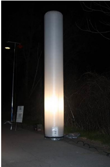
Figure 2-32. Ground mounted cylinder light with 1000 W halogen source.
