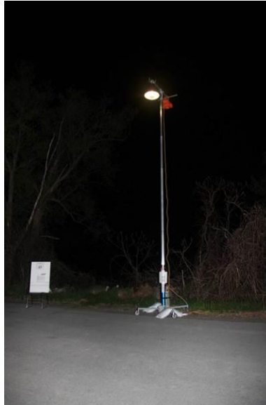
Figure 2-33. Pedestrian light with 25 W remote phosphor LED source.
