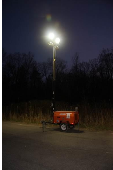
Figure 2-17. Conventional light tower with four 1000 W MH floodlights.
