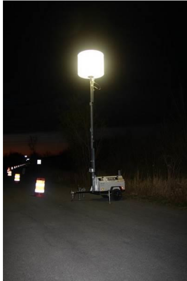
Figure 2-23. Balloon light (internal structure) with four 1000 W MH sources.
