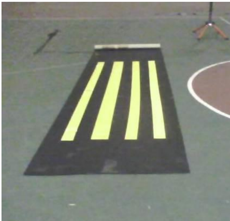
Figure 3-13. Wet reflective temporary lane marking tape (left three segments) and economical grade temporary marking tape (right segment).
