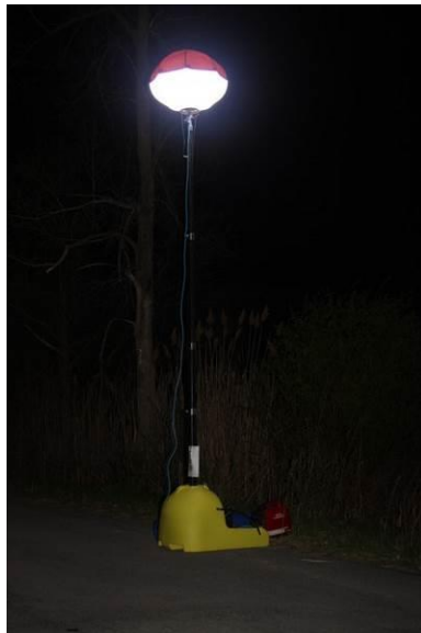
Figure 2-24. Balloon light (umbrella structure) with 1000 W MH source.
