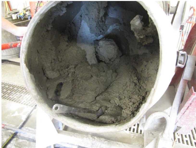
Figure 3.7 – Mortar Mix in Drum Mixer
