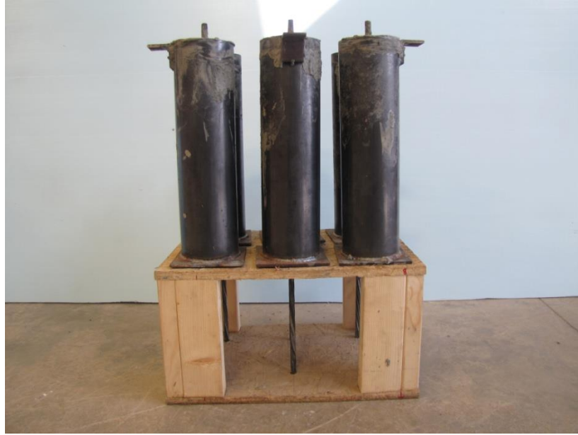
Figure 3.10 – NASP Mold and Strand Setup
