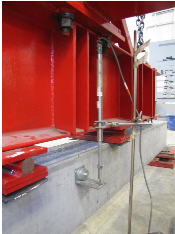
Figure 4.27 – LVDT Setup for Measuring Deflection at Midspan
