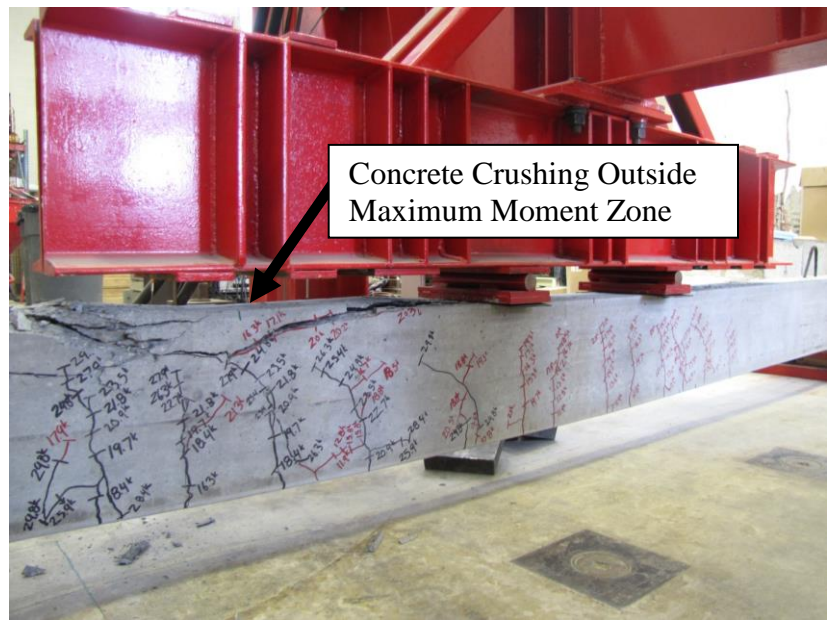
Figure F.15 – S6-2-2_73 at Failure
