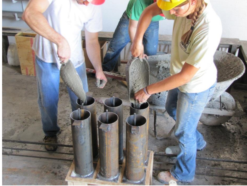
Figure 3.11 – Filling Specimens for NASP Test in Concrete
