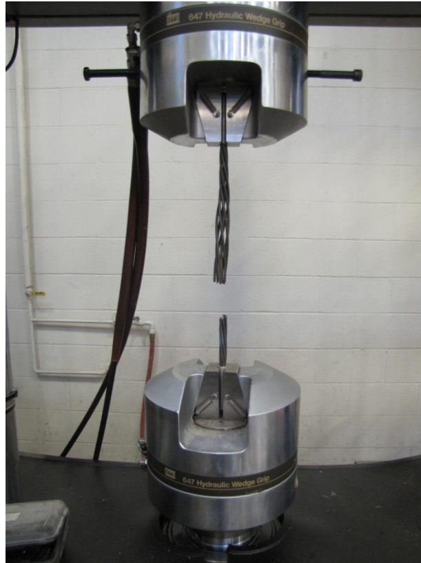
Figure 3.4 – Fractured Tension Test Specimen
