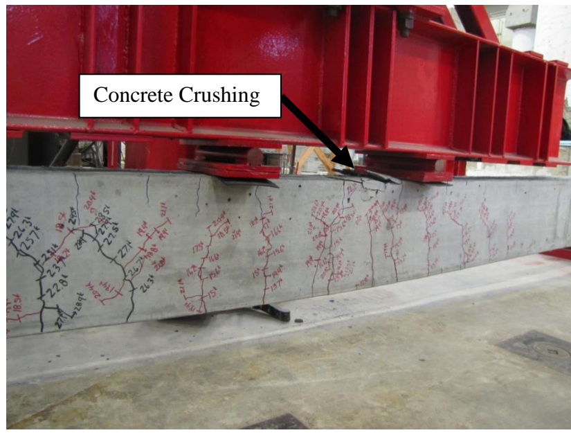
Figure F.31 – S10-2-2_73 at Failure
