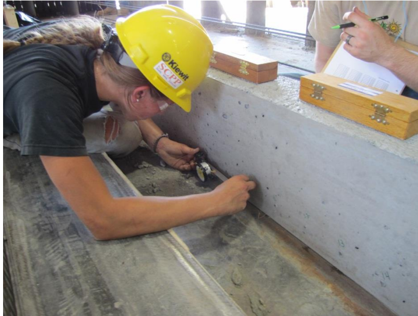
Figure 4.13 – Taking DEMEC Readings
