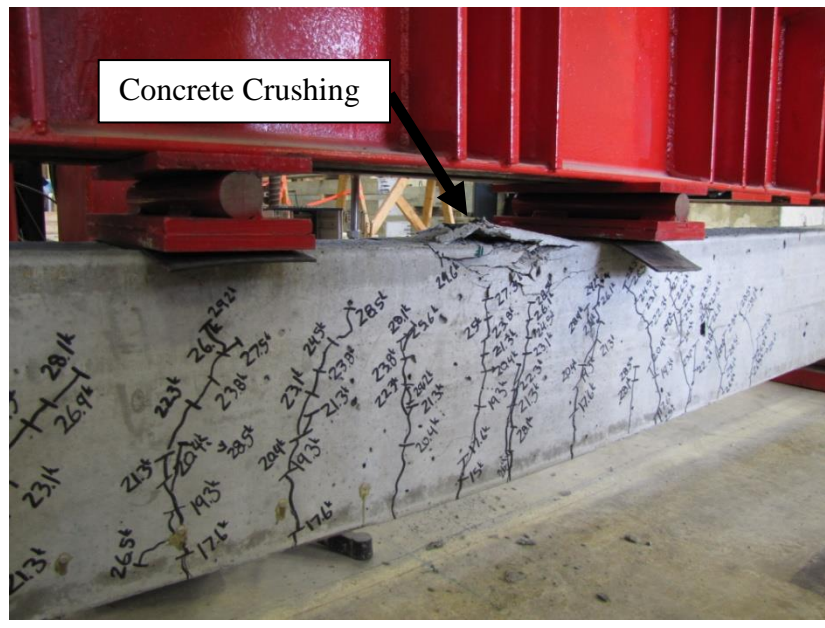
Figure F.21 – C10-2-2_58 at Failure
