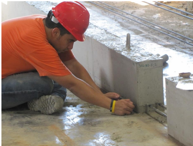
Figure 4.11 – Setting DEMEC Points with Setting Bar
