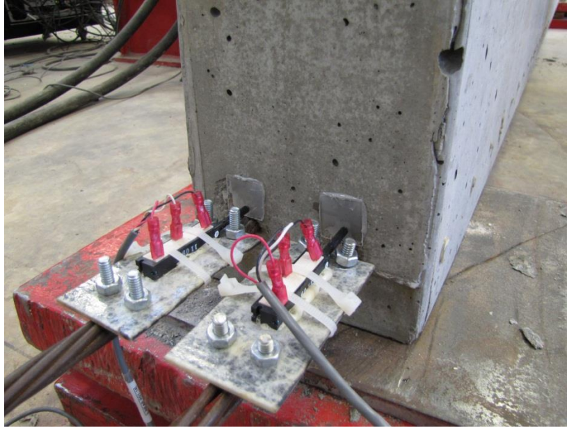
Figure 4.28 – Linear Potentiometer Setup on Four-Point Loading Tests
