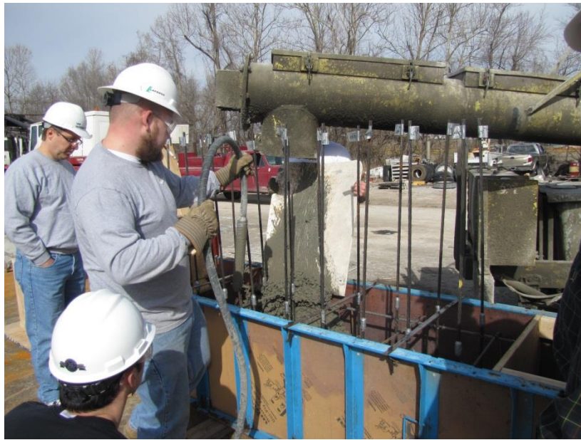
Figure 3.23 – Casting the LBPT Specimen
