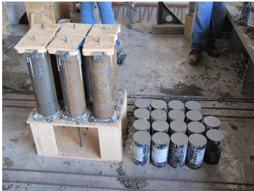
Figure 3.12 – Capped NASP in Concrete Specimens and Cylinders
