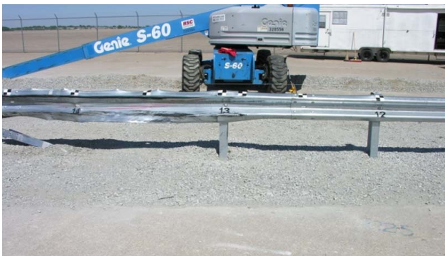
Figure 41. Guardrail Damage between Post Nos. 13 and 17, Test No. MGSNB-1
