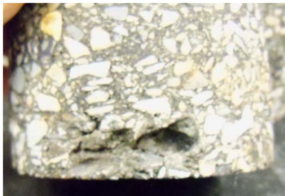
FIGURE 3 Sample that shows significant degradation after MIST conditioning.
