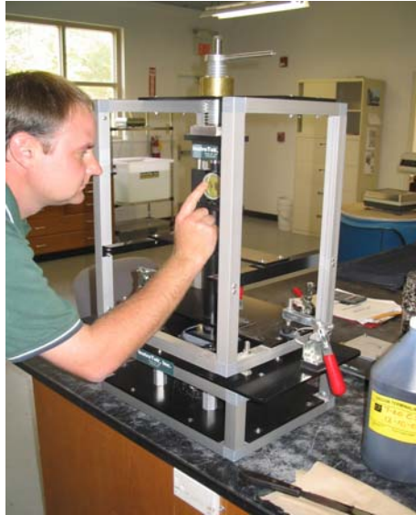
Figure 9. ATACKER™ Device for Tack Coat Bond Strength
