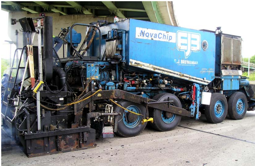
Figure 28. Novachip Spreader Equipped with Tack Tank and Application System
