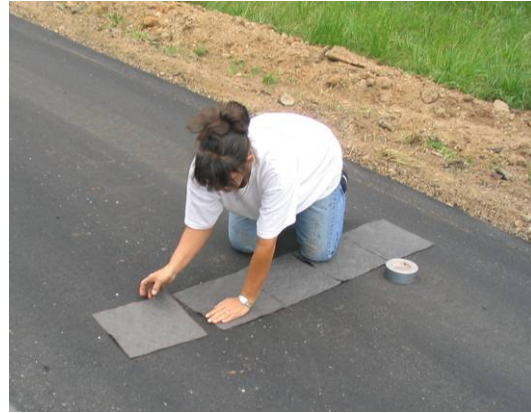
Figure 20. Placing Pads for ASTM D 2995
