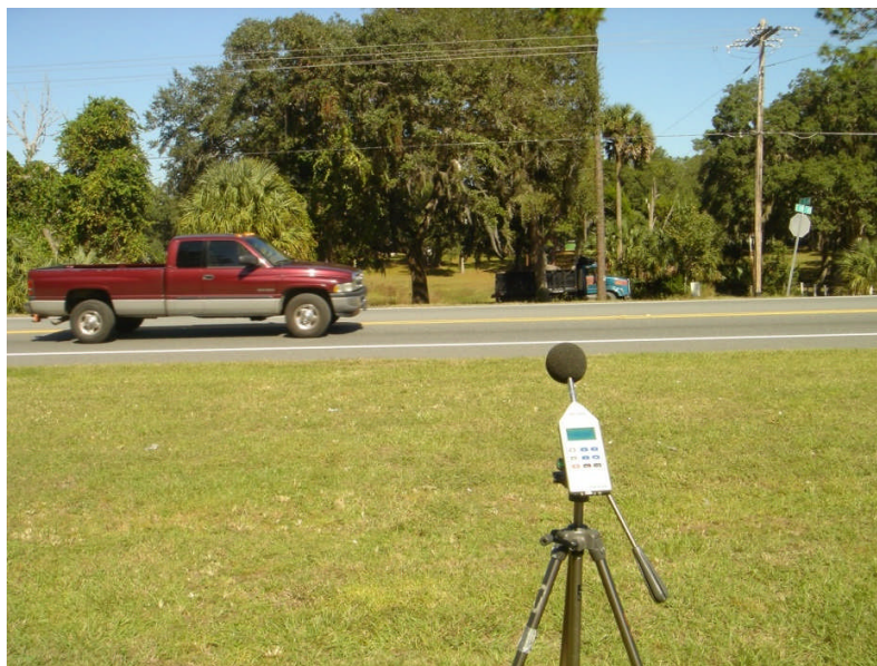
Figure 15. Nearby Passby Microphone Location During Tire/Pavement Test
