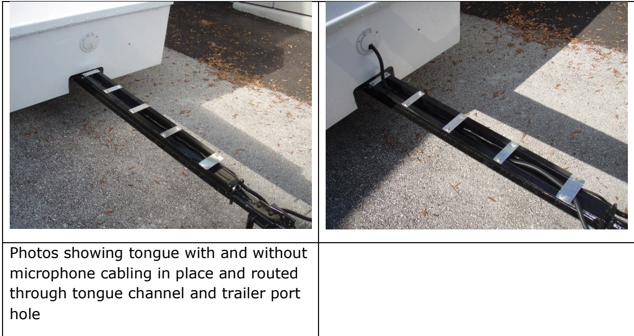
Figure A.1.7. Cable routing on tongue of trailer
