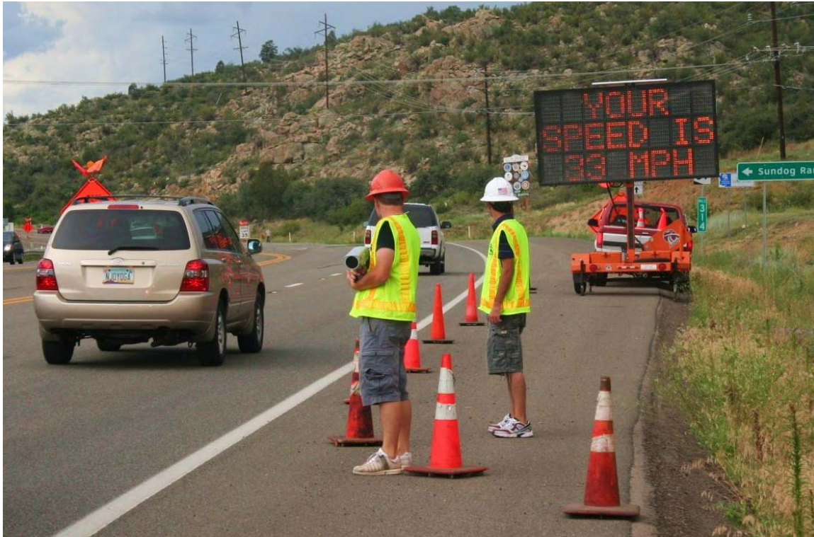
Figure 18. Calibrating the CMSR with a Radar Gun.
