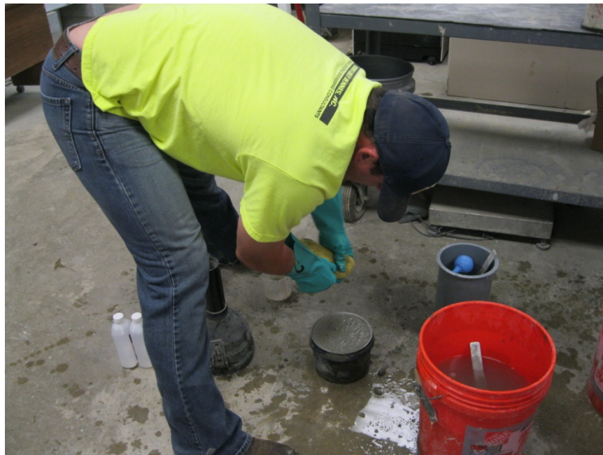
Figure 3 - Air Content Testing
