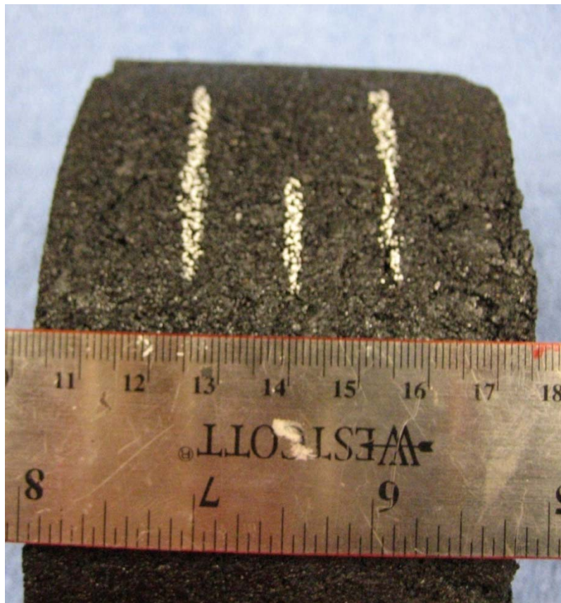
Figure 2.2: Gyratory Compacted Sample Marked for Cutting
