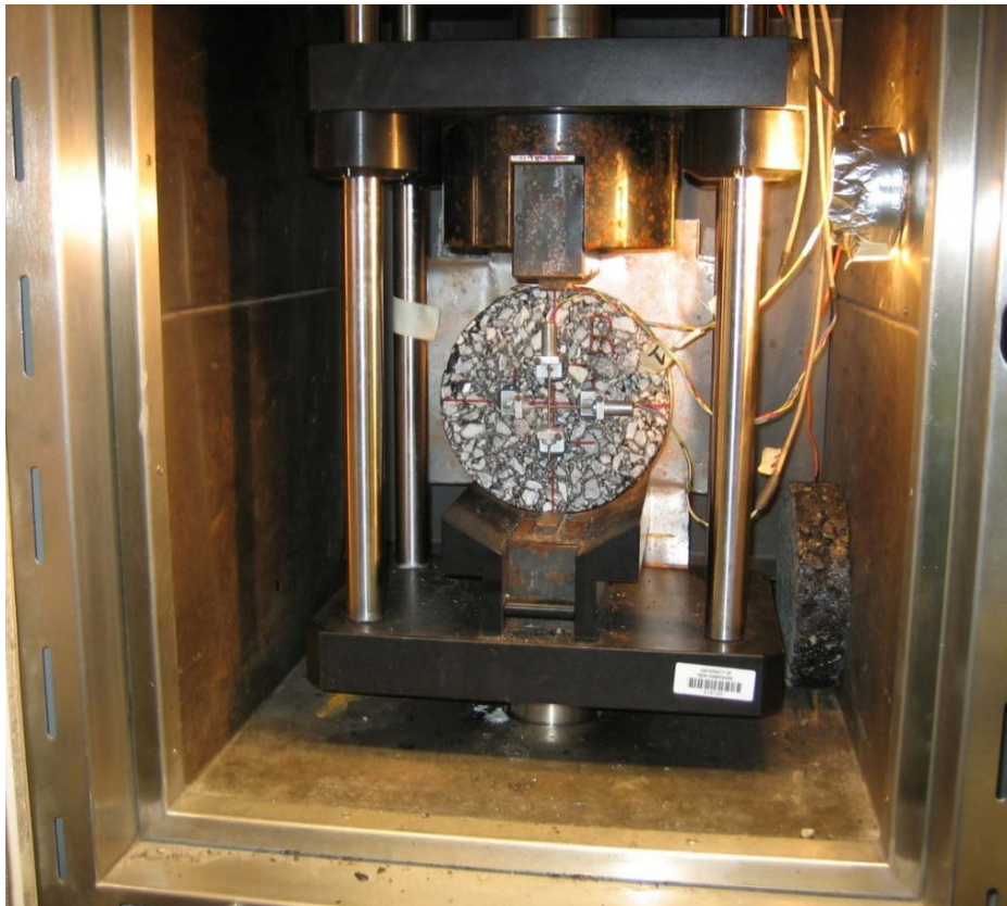
Figure 2.11: Sample and LVDTs in Place and Ready for Testing
