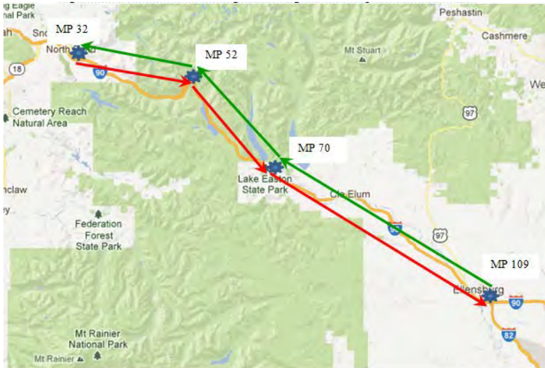
Figure 3-2. Sensor locations and segments along the I-90 Snoqualmie Pass corridor.
