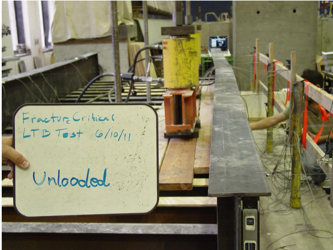
Figure 4-46. Plastic Deformation of Bridge after Load Removal
