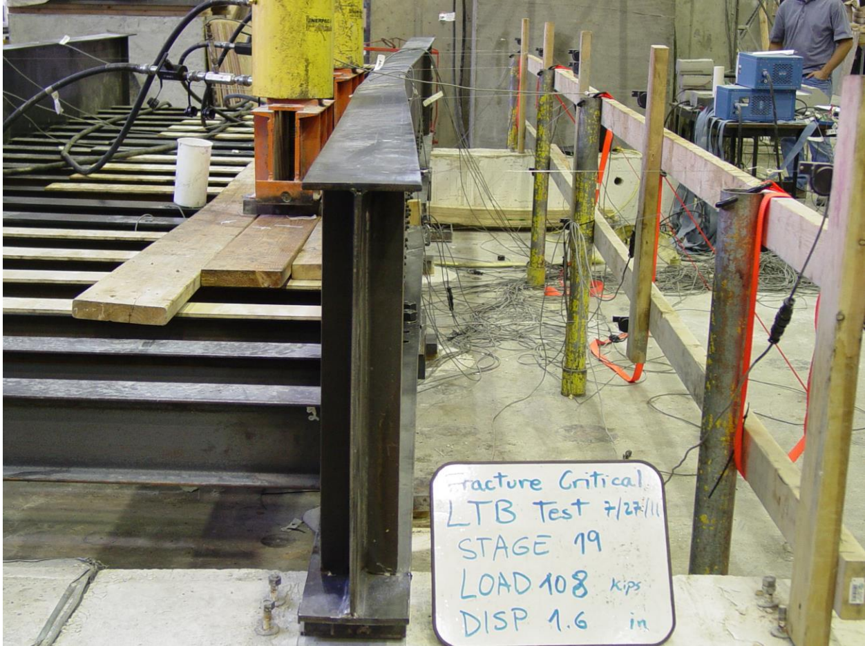
Figure 4-55. Loaded Strengthened Bridge
