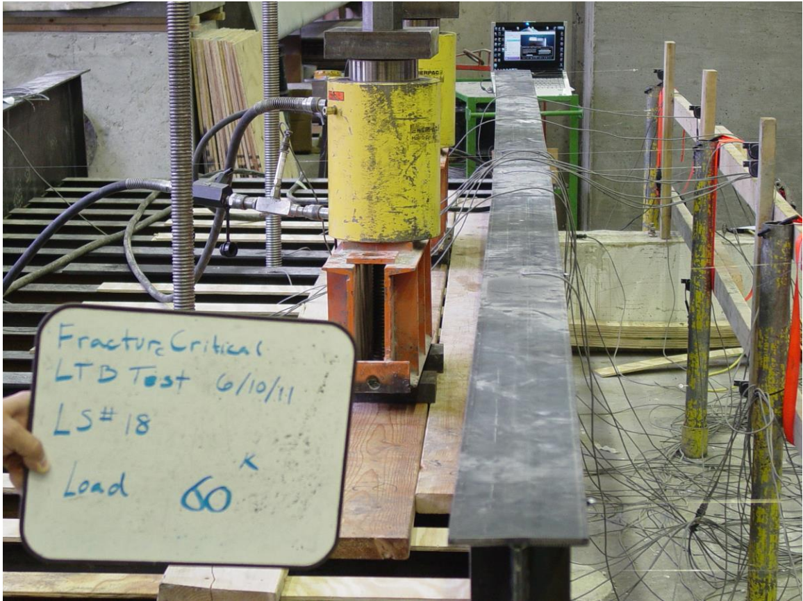
Figure 4-37. Deformed Bridge Under 60 kips of Load
