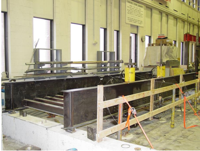
Figure 4-34. Test Bridge Setup Before Loading
