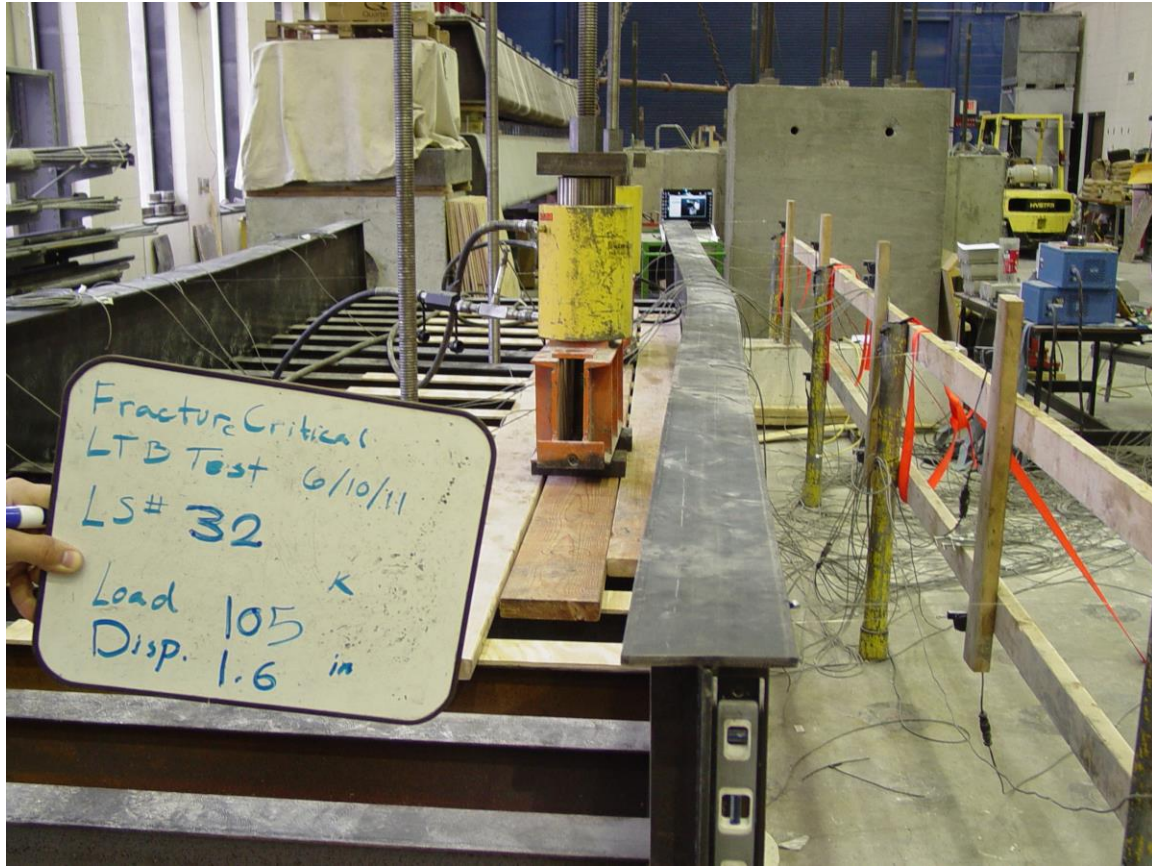
Figure 4-44. Deformed Bridge Under 105 kips of Load
