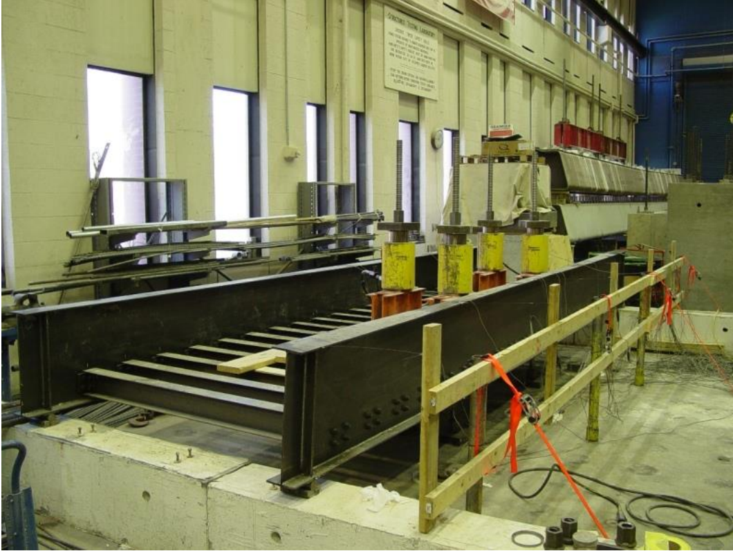
Figure 4-22. Test Bridge with Deep Girders (Initial Trial Loading Configuration)
