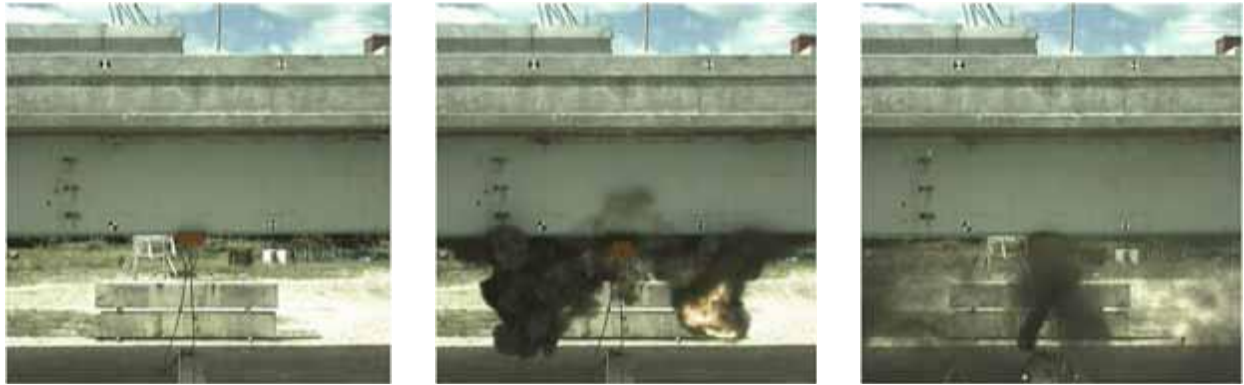
Figure 1-2. FSEL First Bridge Fracture Test [Source: FHWA Report No.: FHWA/TX-10/9-5498-1]
