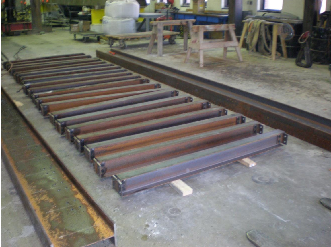
Figure 4-3. Girders and Floor Beams Ready for Assembly
