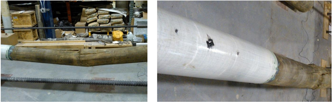
Figure 5.11: Failure of specimen 5 (2 inch deep damage filled with resin + gravel)
