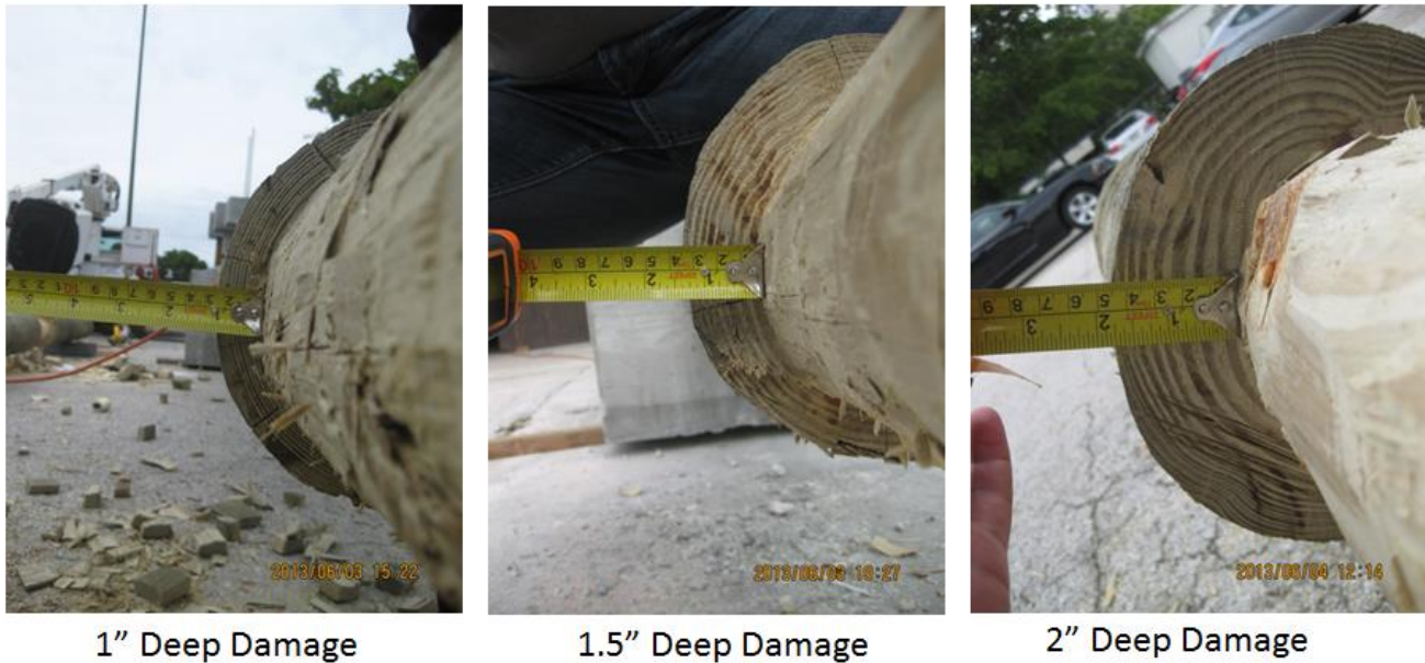
Figure 5.3: Different levels of damage in timber pile test specimens
