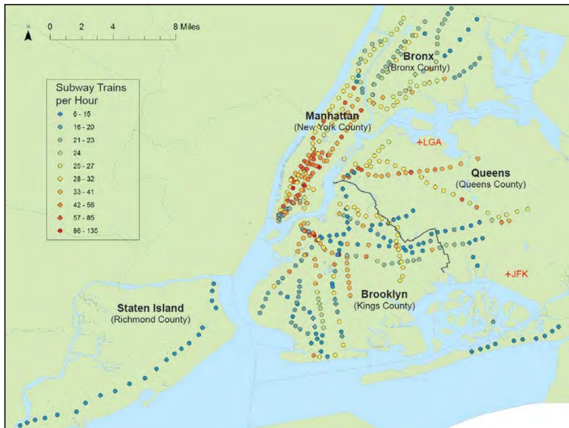
Figure 4. Frequency of Subway Service at Each Station in New York City Between 5:00 p.m. – 6:00 p.m.
