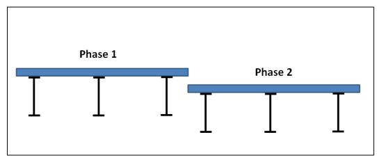
Figure 1-6. Exaggerated differential displacement between phases
