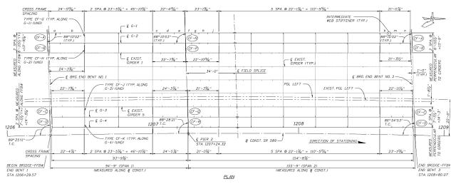
Figure 6-2. Framing plan of the SR-589 Bridge over Hillsborough Avenue
