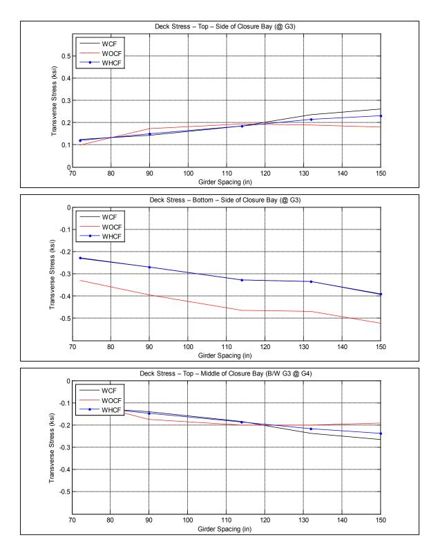
Figure A-6. Transverse deck stresses at middle and side of closure pour vs. girder spacing for bridge I-95 over SR-421
