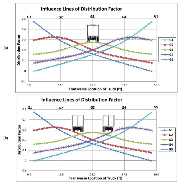
Figure 3-4. The critical positioning for obtaining the distribution factor with: (a) A single truck, (b) Two tracks, (c) Three trucks, (d) Four trucks
