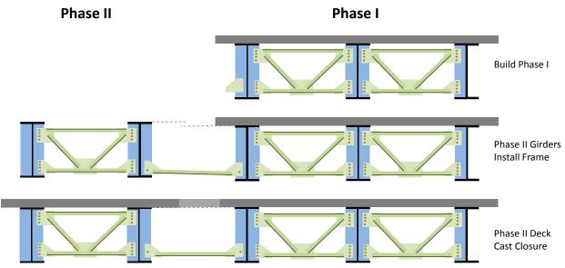
Figure 5-3. Horizontal struts between construction phases
