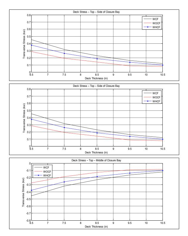
Figure A-47. Transverse deck stresses at middle and side of closure pour vs. deck thickness for bridge SR-589 over Waters Avenue
