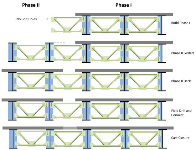
Figure 5-1. Field drilled connection
