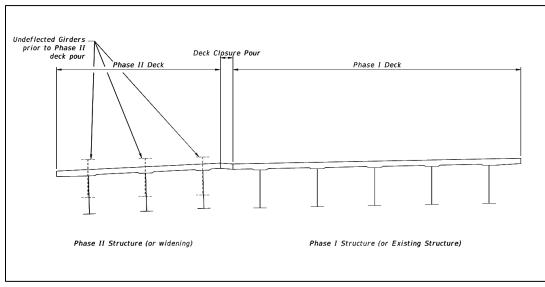
Figure 1-7. Twisting of one phase.
