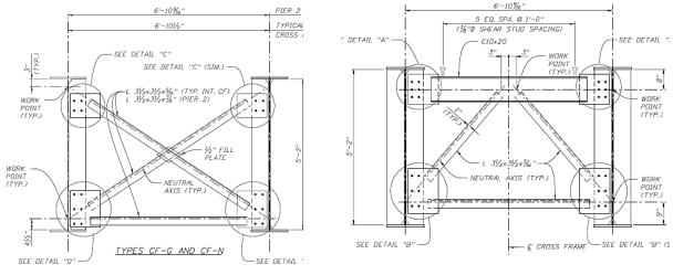
Typical Configuration In-Span
