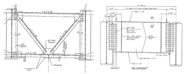
Figure 6-9. Cross-frame details of the SR-589 Bridge over Hillsborough Avenue
