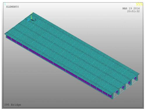
Full Structure Figure 3-1. Finite element model of the bridge I-95 over SR-421
