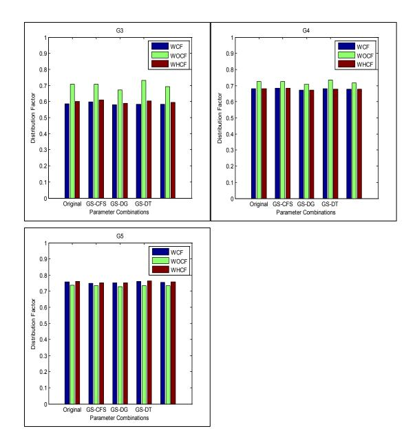
Figure A-34. Distribution factor for girders G3, G4 and G5 related to different Parameter combinations for bridge I-95 over SR-421
