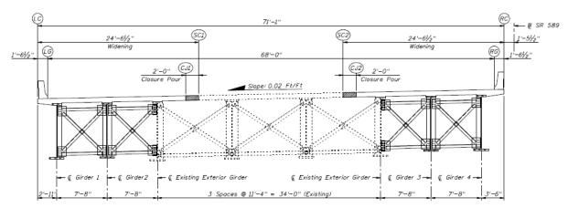
Figure 4-5. Cross-section of the bridge SR-589 over Waters Avenue
