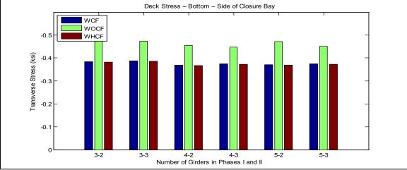
Figure A-31. Transverse deck stresses at middle and side of closure pour vs. number of girders in phases for bridge I-95 over SR-421
