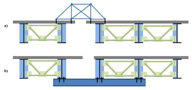
Figure 2-2. Temporary connection between the phases
