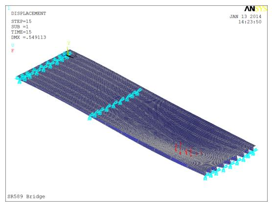
Figure 6-6. SR-589 Bridge over Hillsborough Avenue under truck loading located at critical longitudinal location.
