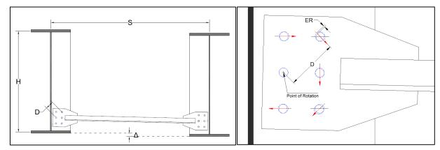
Figure 5-4. Proposed connection detail to accommodate relative vertical displacement
