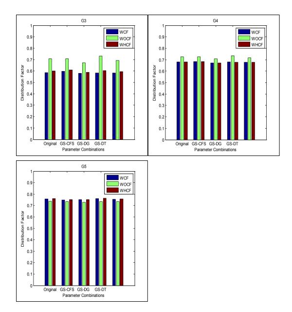
Figure A-66. Distribution factor for girders G3, G4 and G5 related to different parameter combinations for bridge SR-589 over Waters Avenue
