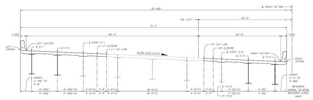
Figure 6-1. Cross-section of the SR-589 Bridge over Hillsborough Avenue
