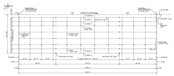
Figure 4-6. Framing plan of the bridge SR-589 over Waters Avenue
