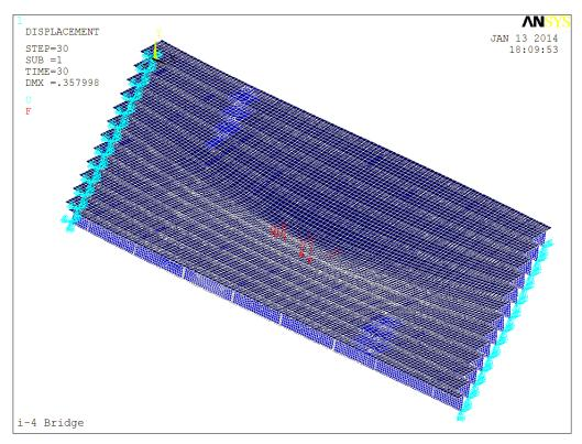
Figure 6-11. Deformed shape of bridge I-4 over SR46 under truck loading located at mid-width and midspan
