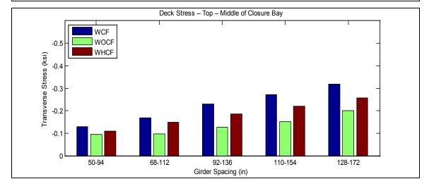
Figure A-42. Transverse deck stresses at middle and side of closure pour vs. girder spacing for bridge SR-589 over Waters Avenue
