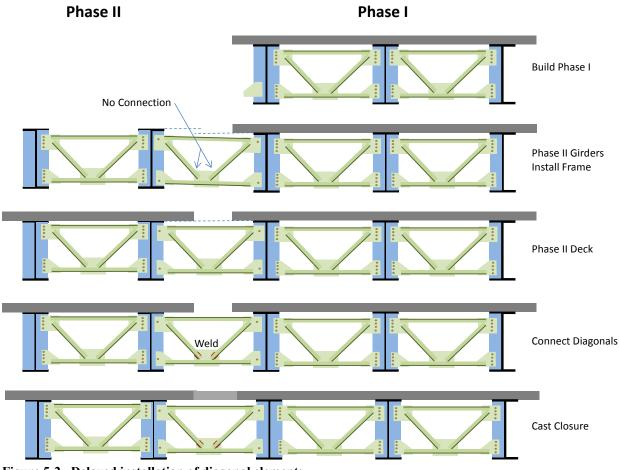
Figure 5-2. Delayed installation of diagonal elements
