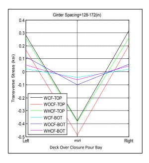
Figure A-40. Transverse stress at closure pour related to different girder spacing for SR-589 over Waters Avenue – Cont'd
