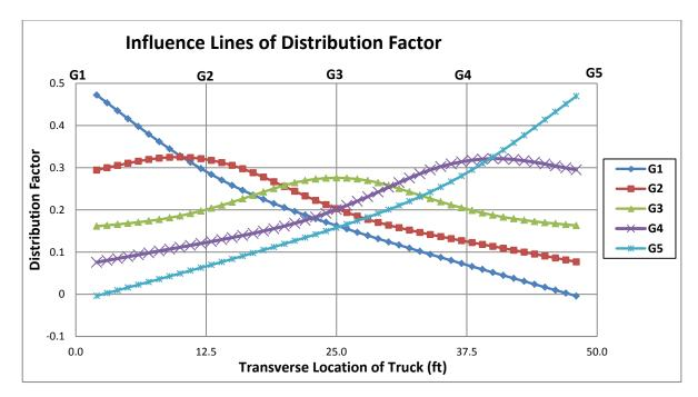
Figure 3-3. Influence lines of distribution factors for all girders, I-95 Bridge over SR-421
