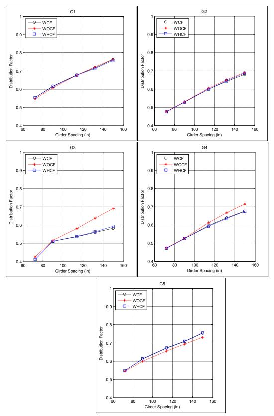
Figure 4-11. Distribution factor vs. girder spacing for all girders of bridge I-95 over SR-421
