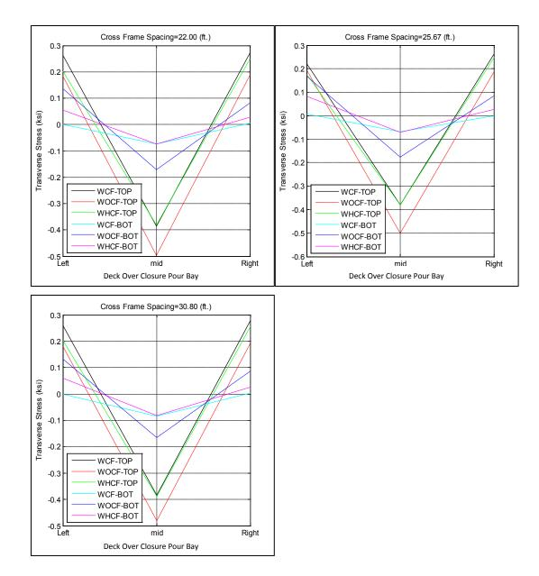
Figure A-22. Transverse stress at closure pour related to different cross frame spacing; 22.0, 25.67 and 30.8 ft. for bridge I-95 over SR-421
