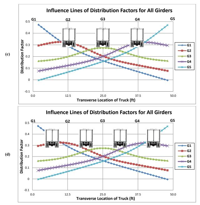
Figure 3-4. The critical positioning for obtaining the distribution factor with: (a) A single truck, (b) Two tracks, (c) Three trucks, (d) Four trucks – Cont'd
