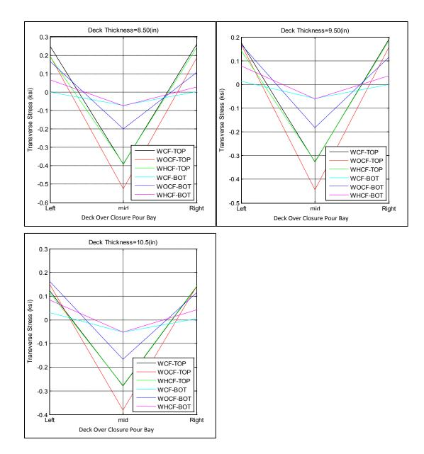
Figure A-10. Transverse stress at closure pour related to deck thicknesses; 8.5, 9.5 and 10.5 inches for bridge I-95 over SR-421
