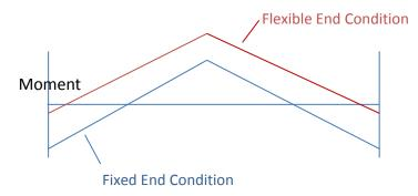
Figure 4-18. Difference moment distribution due to different end flexibility condition.
