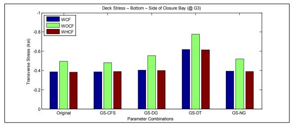
Figure A-36. Transverse deck stresses at middle and side of closure pour vs. parameter combinations for bridge I-95 over SR-421
