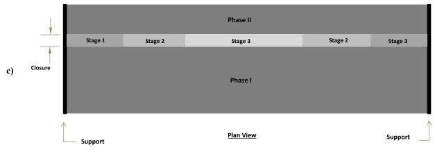
Figure 2-3 Staged casting of closure region
