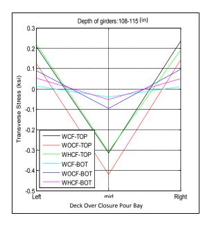
Figure A-50. Transverse stress at closure pour related to different depth of girders for SR-589 over Waters Avenue – Cont'd
