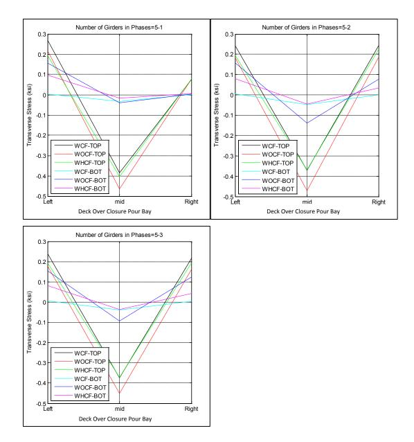
Figure A-30. Transverse stress at closure pour related to different number of girders in phase I and II; 5-1, -5-2 and 5-3 for bridge I-95 over SR-421
