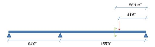
Figure 6-5. Critical longitudinal loading location and corresponding maximum response cross-section for the SR-589 Bridge over Hillsborough Avenue
