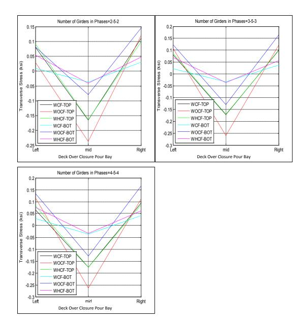
Figure A-62. Transverse stress at closure pour related to different number of girders in phases for SR-589 over Waters Avenue – Cont'd
