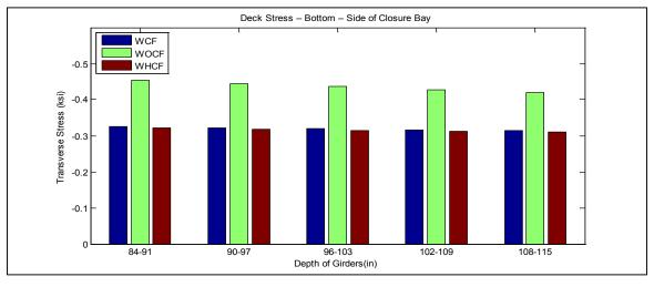
Figure A-52. Transverse deck stresses at middle and side of closure pour vs. depth of girders for bridge SR-589 over Waters Avenue
