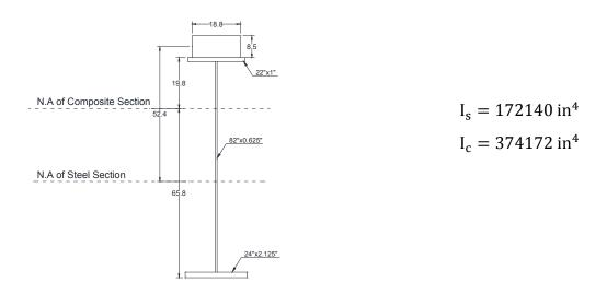
Figure 6-12. Details of steel and composite cross-section
