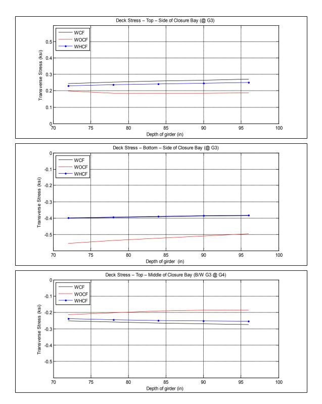
Figure A-18. Transverse deck stresses at middle and side of closure pour vs. depth of girders for bridge I-95 over SR-421
