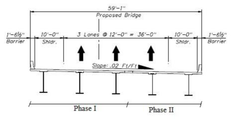
Figure 4-1. Cross-section of the bridge I-95 over SR-421
