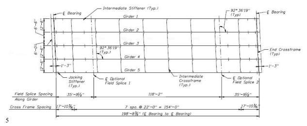
Figure 4-2. Framing plan of the I-95 Bridge over SR-421
