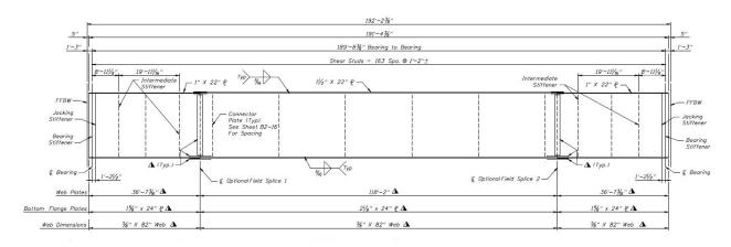
Figure 4-4. Typical details of girders of the I-95 Bridge over SR-421
