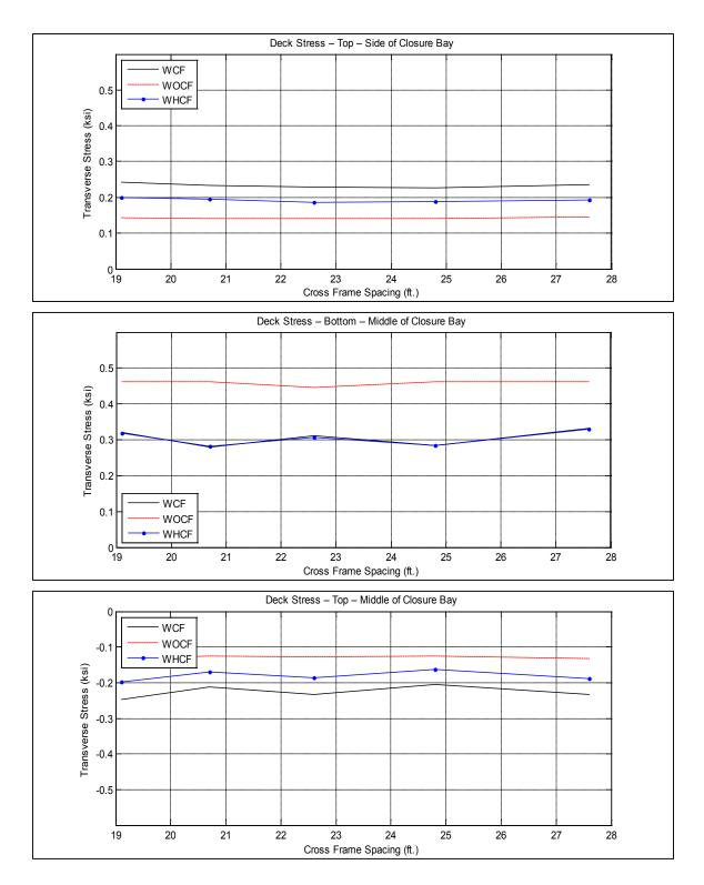
Figure A-57. Transverse deck stresses at middle and side of closure pour vs. cross-frame spacing for bridge SR-589 over Waters Avenue
