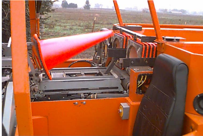
Figure 2-13 Stowage system operating without covers
