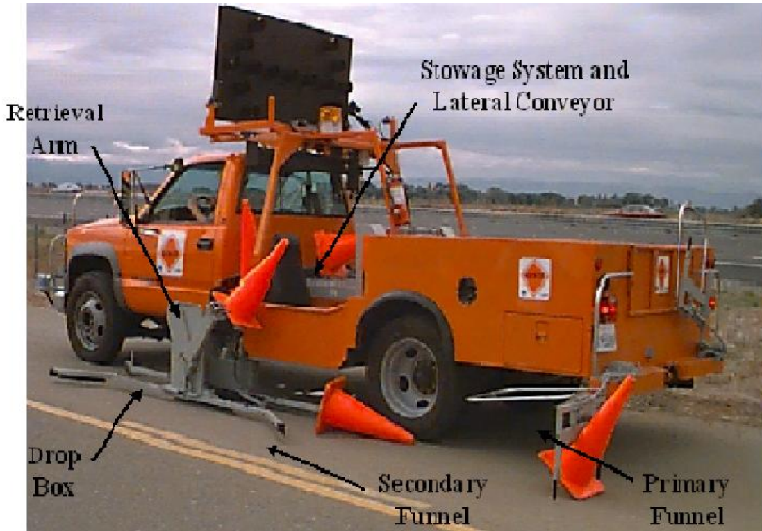
Figure 2-1 The AHMCT Automated Cone Machine ACM-1
