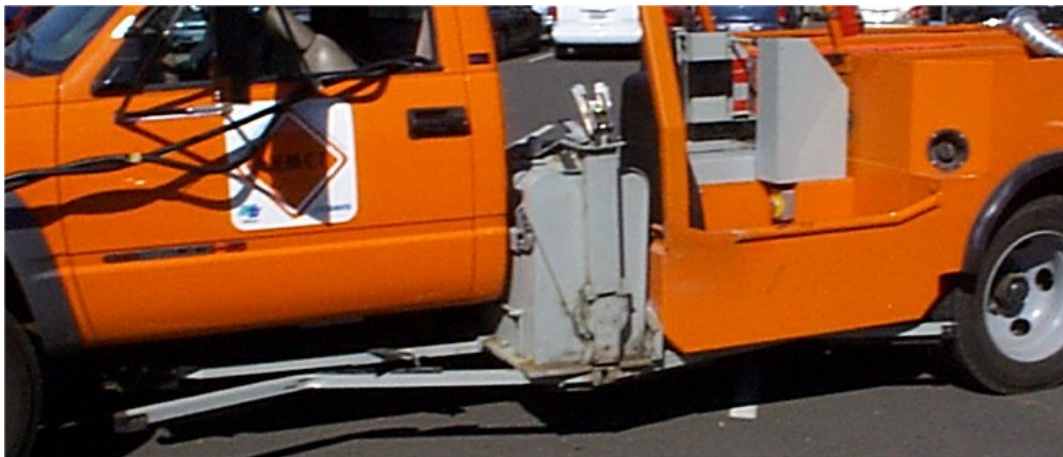
Figure 2-18 Stowed drop box system and retrieval arm (Left side)
