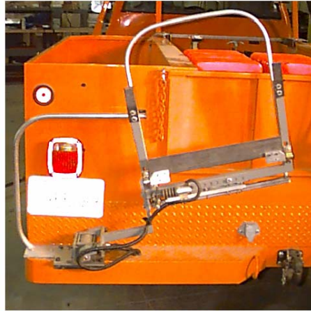
Figure 2-20 Retracted primary funnel system
