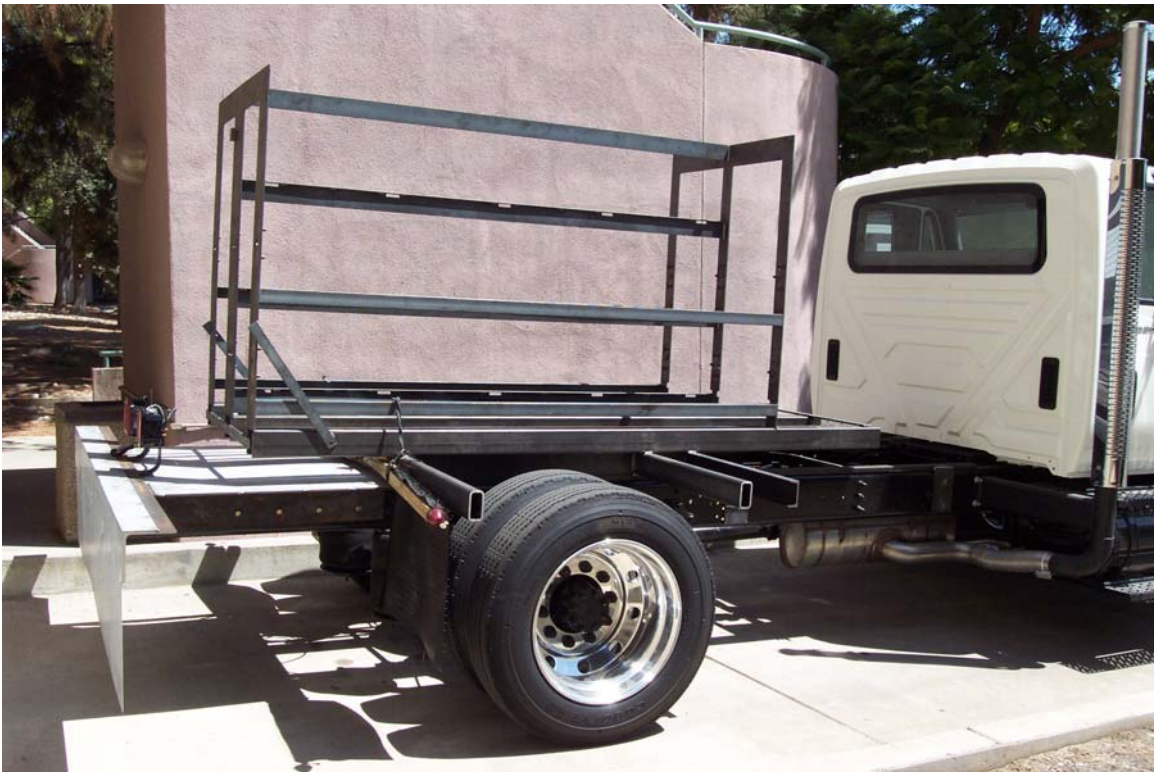
Figure 4-12 Storage framework before attachment of panels
