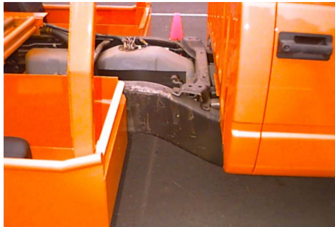
Figure 2-2 Cone truck with cone body moved rearward
