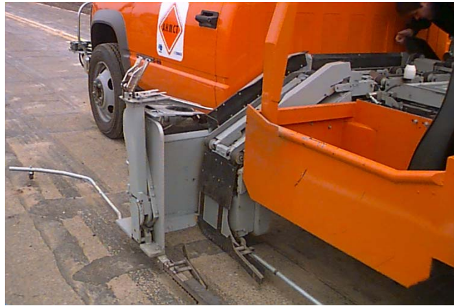
Figure 2-16 Drop box system (Left side)
