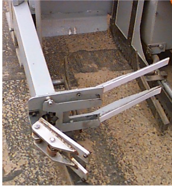
Figure 2-17 Retrieval arm in cone retrieval position
