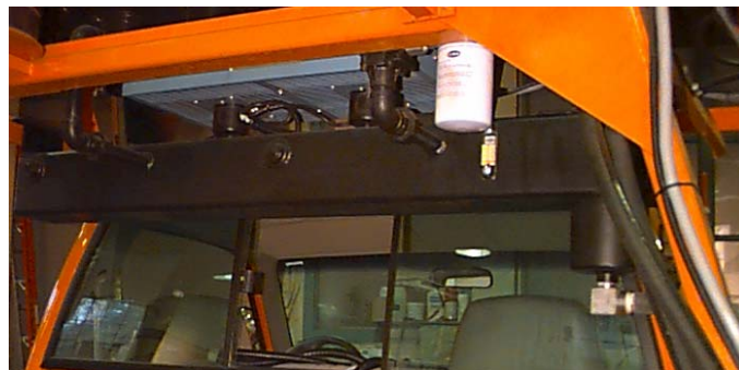
Figure 2-23 Hydraulic fluid reservoir and heat exchanger
