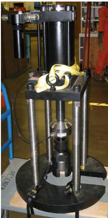
Figure 5-1: 267 kN (60 kip) Load Frame
