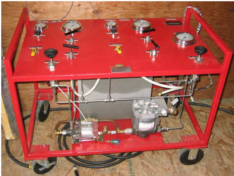
Figure 5-6: Air Powered Pump
