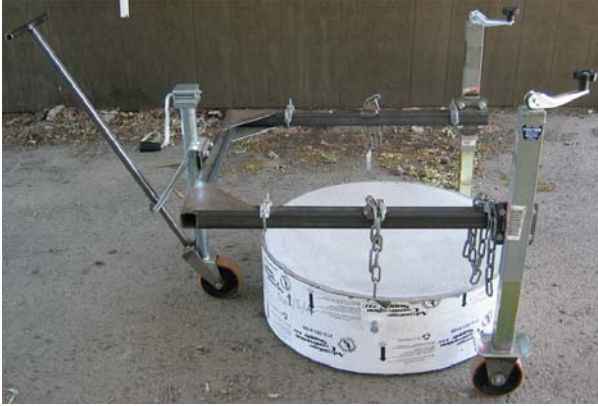
Figure 5-7: Concrete Cylinder Mover
