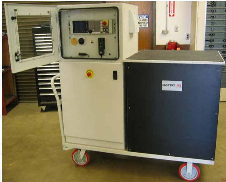
Figure 5-2: Cart with Controller and Hydraulic Pump
