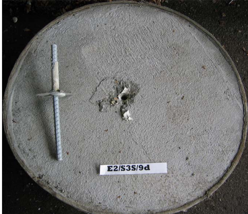
Figure A-3: Typical Concrete/Adhesive Interface–Adhesive/Rebar Interface Failure
