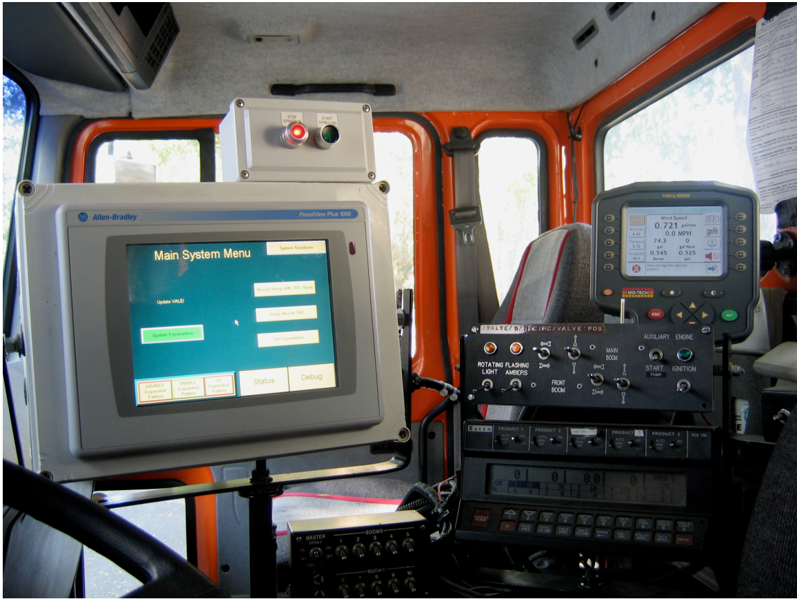
Figure 4. Driver view inside cab of spray vehicle containing IHAS operator interface with touch-panel (left), emergency stop switch (above touch-panel) and global positioning system (right) installed adjacent to conventional spray control systems.
