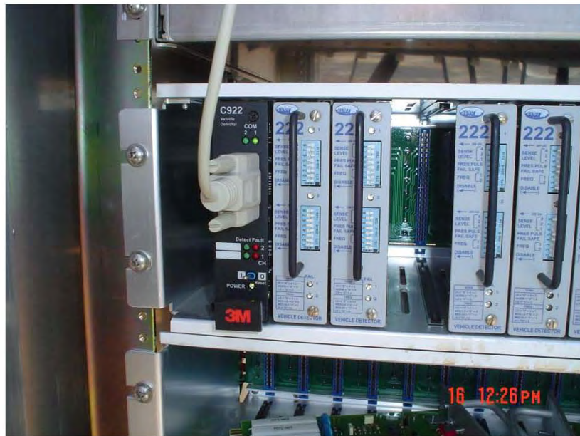
Figure 2.7. Laptop using RS232 serial interface with C922 3M Canoga Card
