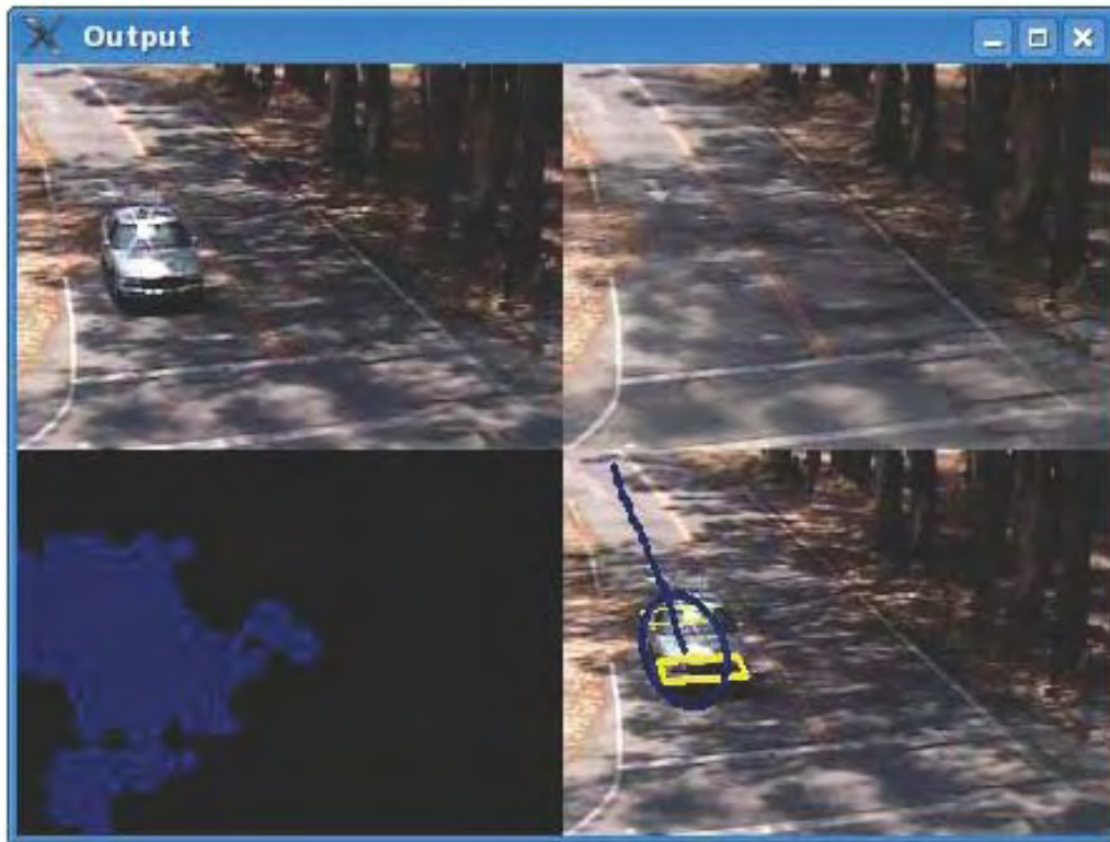
Figure 2.13. Vehicle tracking with virtual loop matched with real loop on the ground
