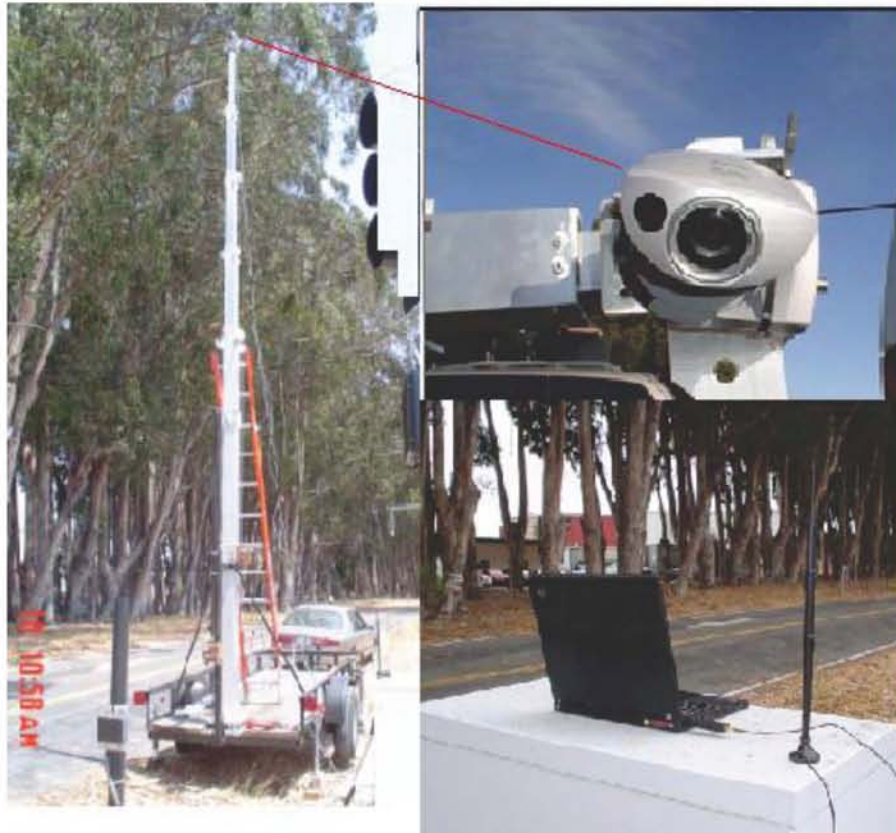
Figure 2.5. Video Camera Mounting on Mobile Trailer: Left: Mobile retractable pole; Upper right: PTZ camera on top for looking at the loop and for vehicle tracking to obtain baseline data; Lower right: video computer also run IEEE 802.11b wireless communication via USB port.
